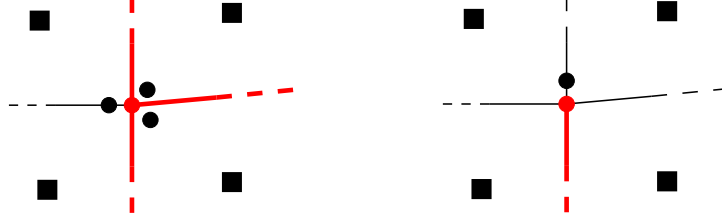
Figure 2.5: Zoom on the fracture intersection for three fractures (left) and on the fracture tip for one immersed fracture (right). Illustrated are four cells (indicated as boxes) and the d.o.f. at the singular point for the discontinuous hybrid-dimensional models (interfacial d.o.f. in black and fracture d.o.f. in red).
