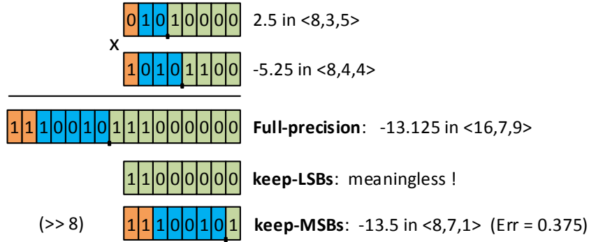
Figure 5.5 – Fixed-point multiplication example.
