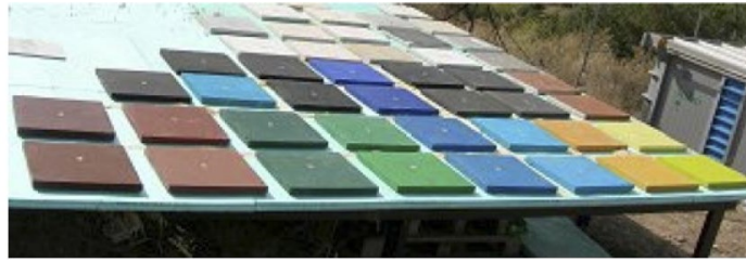
Figure 3. 29: The tested samples placed on the modulated horizontal platform
