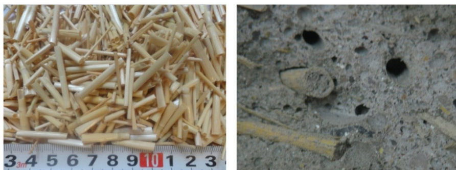
Figure 3. 41: Barley straws with concrete
