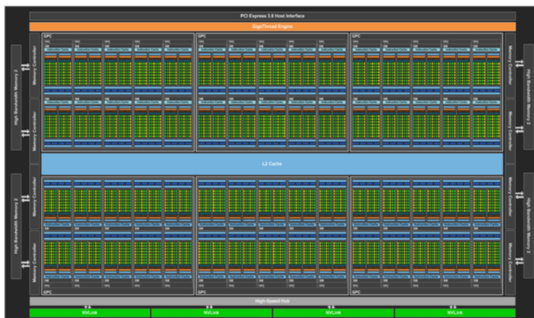
Figure 1.5: A block diagram of Nvidia's Pascal GPU
