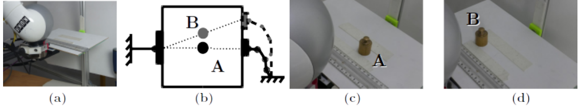
Figure 4.42: Co-manipulation for keeping the balance: a - the robot arm holding a plate that rotates around its center, b - illustration of the changes of the center of mass of the plate from point A to B, c - a scale-weight is placed on the plate at point A, d - the scale-weight is placed at point B.
