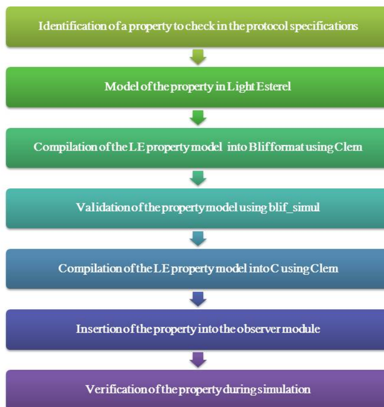
Figure 3.9: The different stages used for property verification in SNOOPS.
