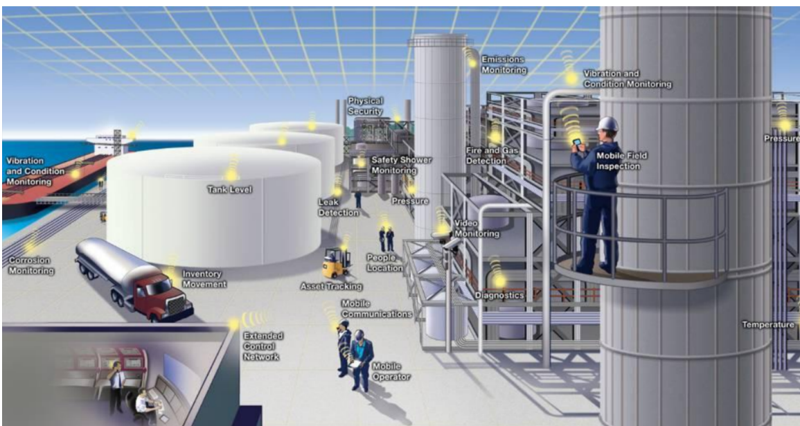
Figure 1.3: Applications of industrial WSN in a factory (source: [10]).
