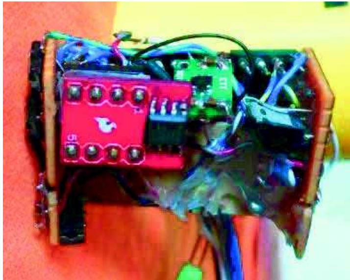
Figure 5.4 A wired prototype with FRAM memory and IMU. The horizontal length of the device in the figure is approximately 40 mm.
