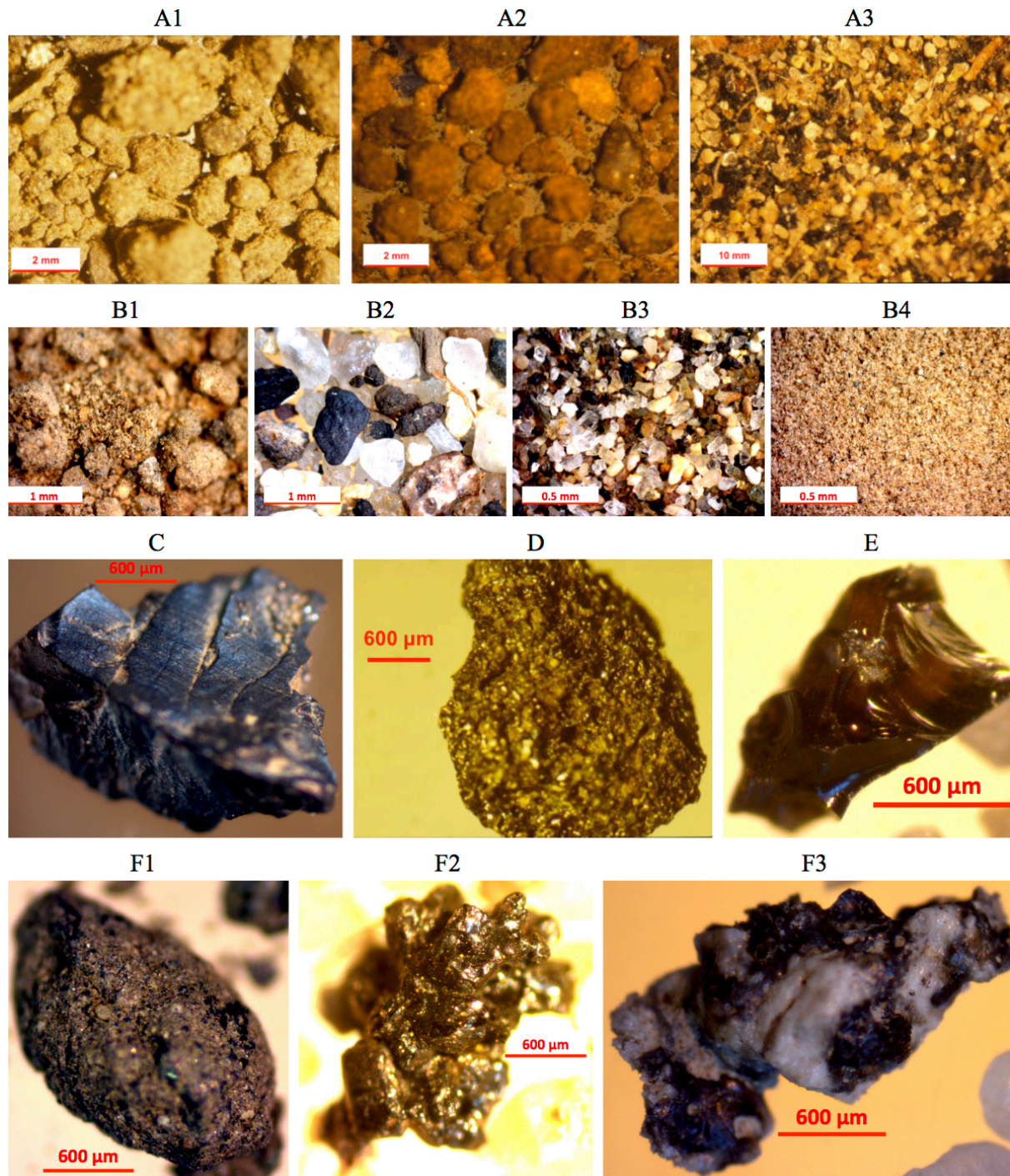
Figure 2.1. Stereomicroscopic pictures. A1: VS soil untreated; A2: VS soil acetone-treated; A3: VS soil fully oxidized; B1: IdF soil untreated; B2: 200-2000 \mu\text{m} fraction of IdF soil; B3: 63-200 \mu\text{m} fraction of IdF soil; B4: <63 \mu\text{m} of IdF soil; C: coal particle (from IdF); D: coke particle (from VS); E: glassy slag particle (from NoF); F: solid aggregates of resinified/weathered tar oil and embedded soil particles (F1: from VS, F2: from IdF, F3: from Michle).
