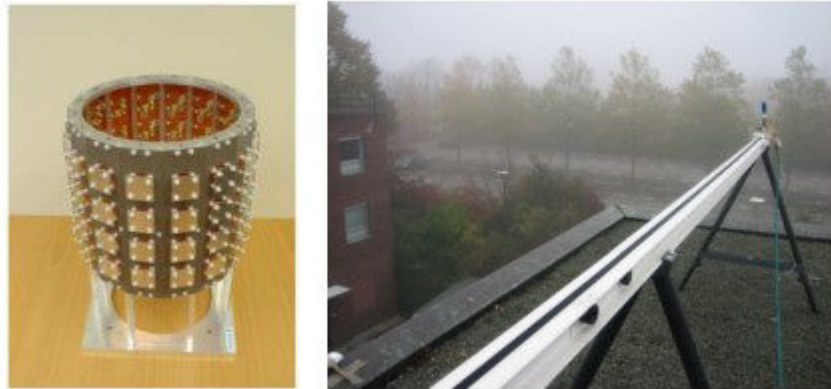
Figure 2.6.4 Two large antenna arrays at the base station side: on left: a cylindrical array with 128 patch antenna on right: a virtual linear array with 128 omnidirectional antenna positions [26].
