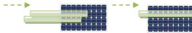
Fig. 3.7: Shading nine cells from: (i) two different lines (9 cells/ P), and (ii) nine cells from the same line (9 cells/ S).
