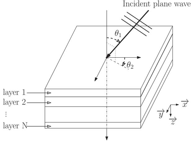
FIGURE 5. Multilayered system studied under plane wave incidence.
