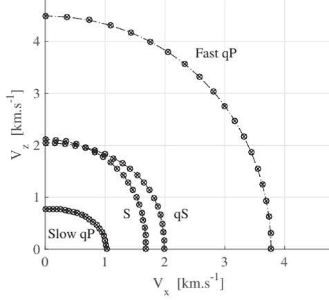
FIGURE 1. Phase velocities of the waves in the  $xz$ -plane of a human femoral bone at  $f = 10$  kHz. Circled dashed line: method proposed by Carcione<sup>11</sup>. Crossed dotted line: semi-analytical method proposed by Parra Martinez *et al.*<sup>44</sup>
