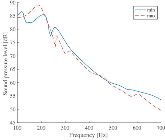
FIGURE 10. Sound pressure level spectra for maximum and minimum solutions of the optimisation problem defined by Lind Nordgren *et al.*<sup>34</sup>, computed with the method proposed in Chap. II.
