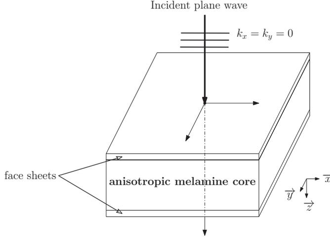
FIGURE 11. Multilayered system setup used in the optimisation problems.
