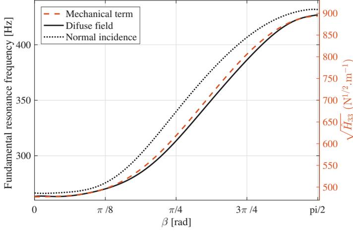
FIGURE 8. Fundamental resonance of the multilayered system under normally incident and diffuse field excitations, and stiffness coefficient  $\sqrt{H_{zz}}$  as a function of the material alignment rotation.
