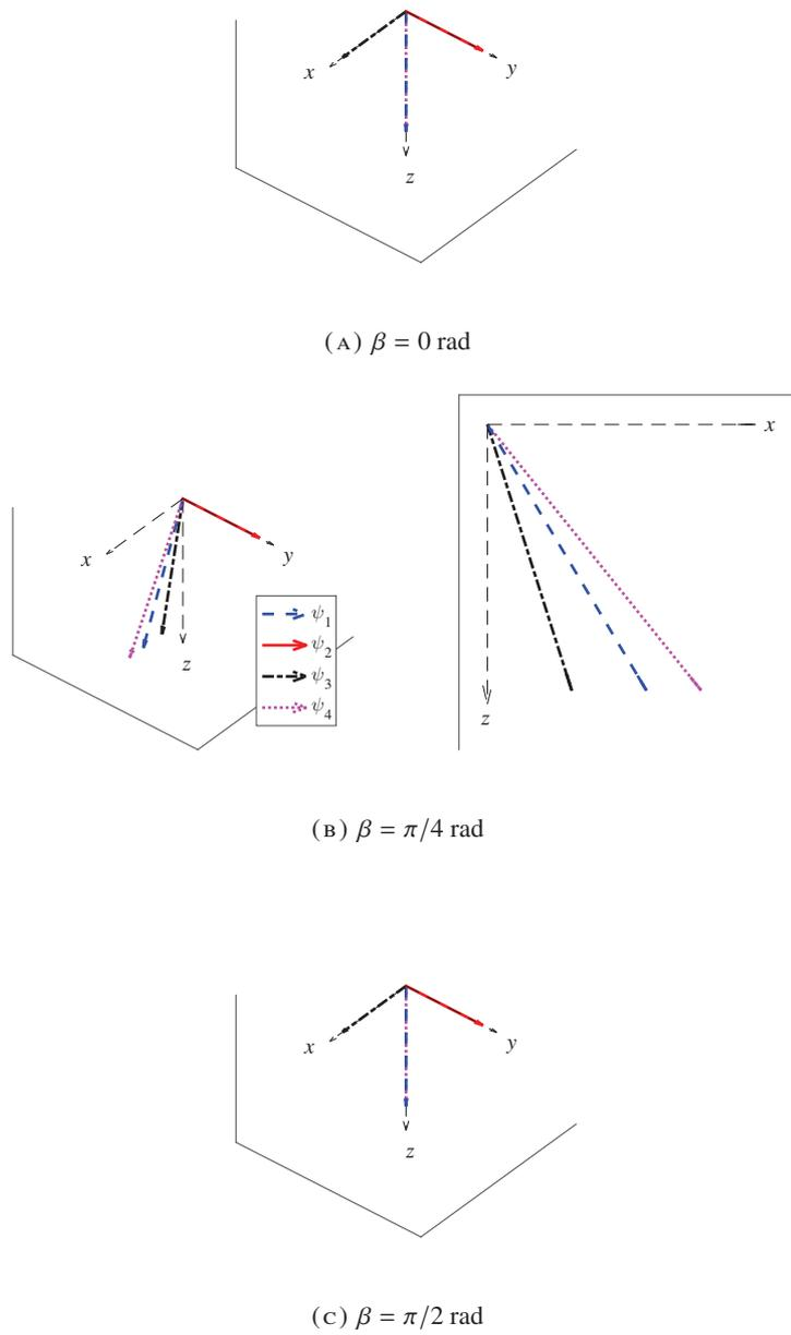
FIGURE 3. Wave polarisations in terms of normalised displacement of the solid phase of the melamine foam at  $f = 100$  Hz.
