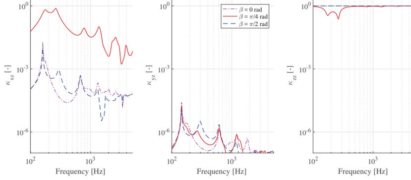
FIGURE 9. Relative deformation of the solid frame of the poroelastic core in the  $xz$ - and  $zz$ - planes, according to Eq. (51), under normally incident plane wave excitation of the panel. The relative deformation in the  $yz$ -plane is negligible in this case.
