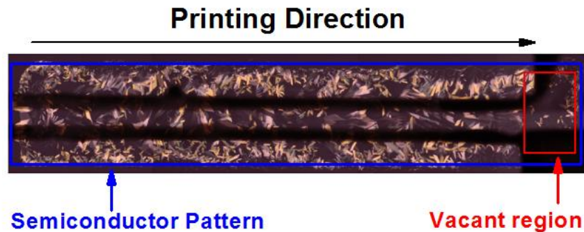
Figure 3-59: Polarized optical picture of fully inkjet printed OTFT
