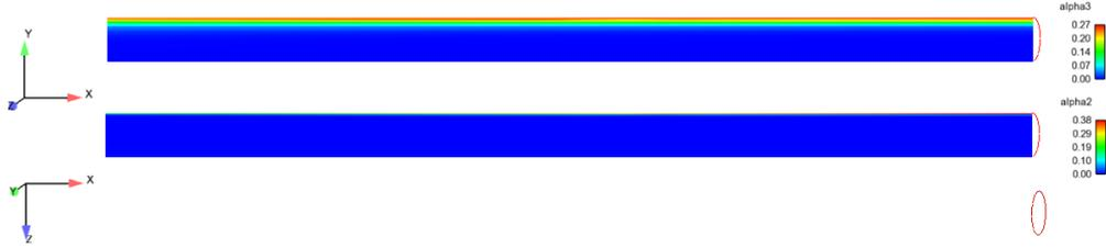
Figure 11.7: Simulation results of the METERO test case with  $J_L = 4.42 \text{ m.s}^{-1}$  and  $J_G = 0.127 \text{ m.s}^{-1}$ , corresponding to a stratified bubbles flow regime, top to bottom: volume fraction of the dispersed gas field (side view), volume fraction of the continuous gas field (side view) and isosurface  $\alpha_{cg} = 0.5$  (top view), the fluid is flowing from the left to the right, RANS model, intermediate mesh.
