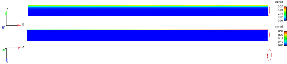
Figure 11.6: Simulation results of the METERO test case with J_L = 2.65 \text{ m.s}^{-1} and J_G = 0.127 \text{ m.s}^{-1} , corresponding to a plug flow regime, top to bottom: volume fraction of the dispersed gas field (side view), volume fraction of the continuous gas field (side view) and isosurface \alpha_{cg} = 0.5 (top view), the fluid is flowing from the left to the right, RANS model, intermediate mesh.
