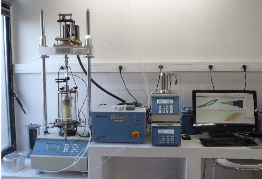
Figure 34. Système triaxial cyclique asservi (Geoslab, 2015)
