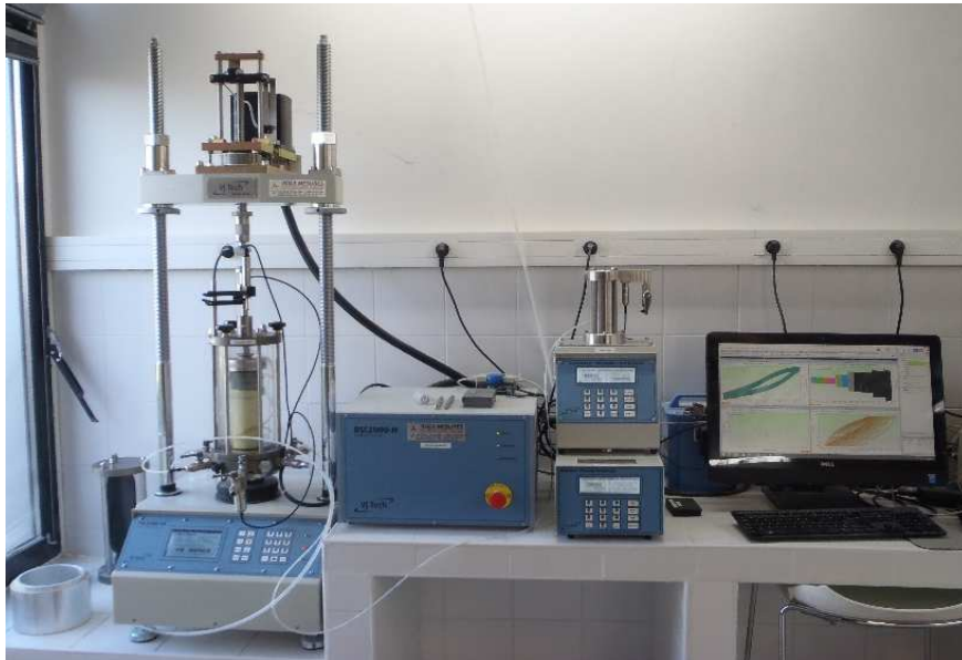
Figure 4.40 Système asservi triaxial cyclique (Geoslab, 2015)
