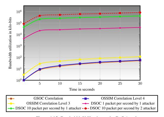
Figure 4.15: Bandwidth Utilization under DoS Attack
