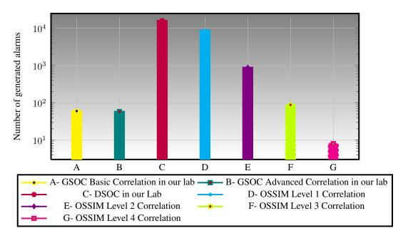
Figure 4.8: GSOC Comparison with OSSIM and DSOC under Brute Force Attack in Our Lab
