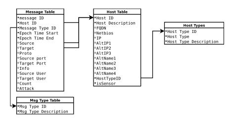
Figure 3.8: Simplified View of the Composition of the Formatted Alert
