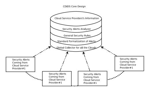
Figure 5.1: Cloud Distributed Intrusion Detection (CDIDS) Core Design
