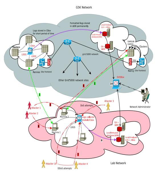
Figure 4.16: Stopping Propagation of Cross-Domain Attacks between Our Lab and G5K Network
