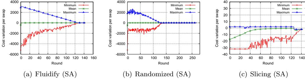
Figure 3.9: Variation of the cost function per swap over time. Lower is better. ( $N = K_0 = 3200$ ,  $k_{\text{net}} = k_{\text{data}} = 16$ , note the different scales) Fluidify (SA) shows the highest amplitude of variations, and fully exploits simulated annealing, which is less the case for Randomized (SA), and not at all for slicing.
