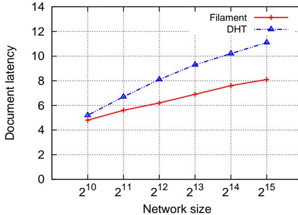
Figure 4.8: Filament vs DHT based on document latency
