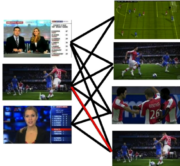
Figure 1.16: The distance between two videos equals to the distance between two most similar keyframes (the red line in this example).
