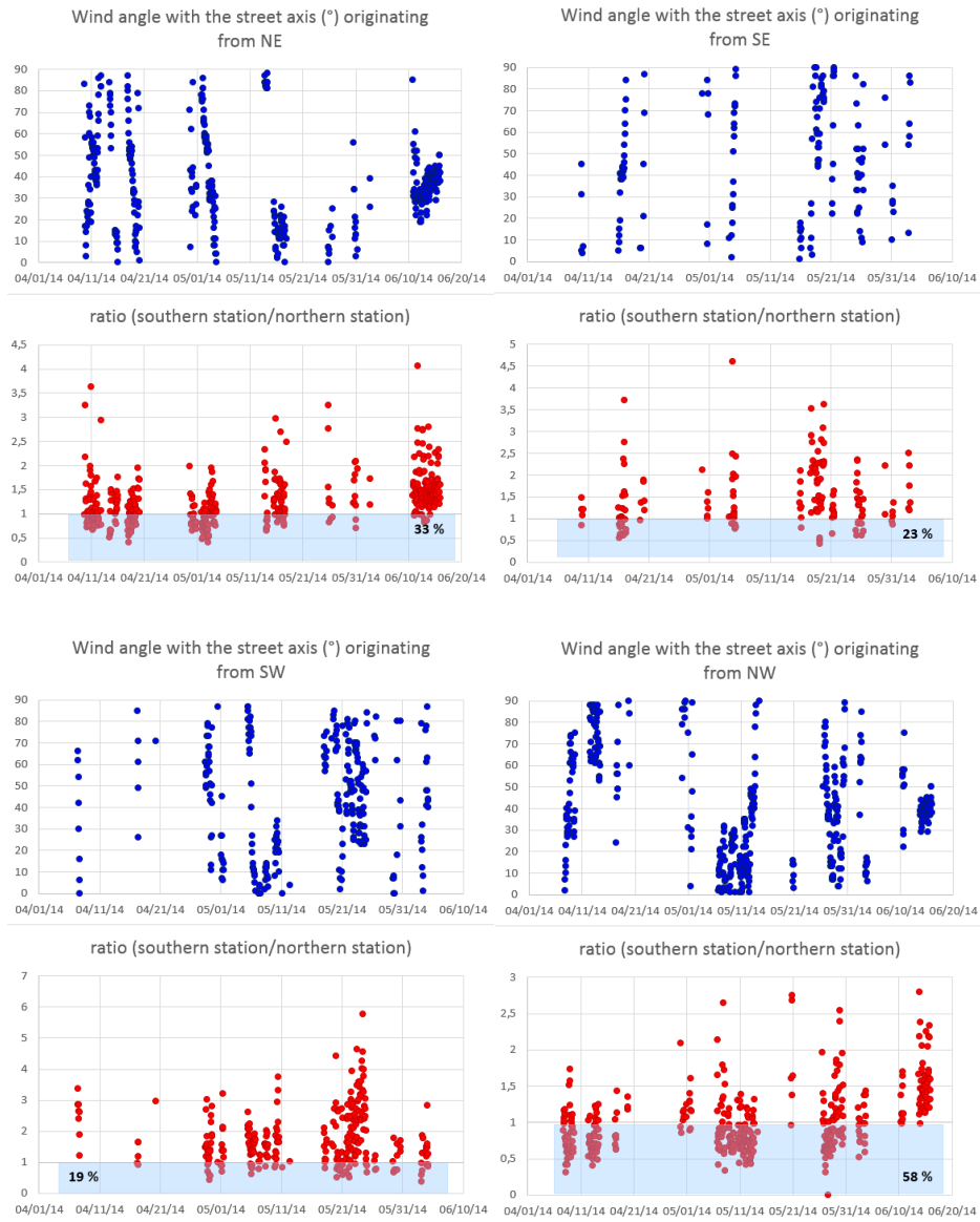
Figure 3.5 - Wind directions according to street axis and its origin by quadrant and the ratio of the southern station (E2) concentration over the northern station (E3) concentration as a function of time. Frequency of ratio lower than 1 is given in %.
