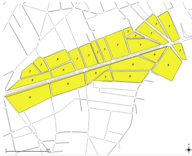
Figure 3.1 - Alsace-Lorraine district geometry (2D view) as it is taken into account in SinG (view limited to the area around the boulevard) with building heights in meter based on IGN database and roads based on data from the SymuVia traffic simulation.
