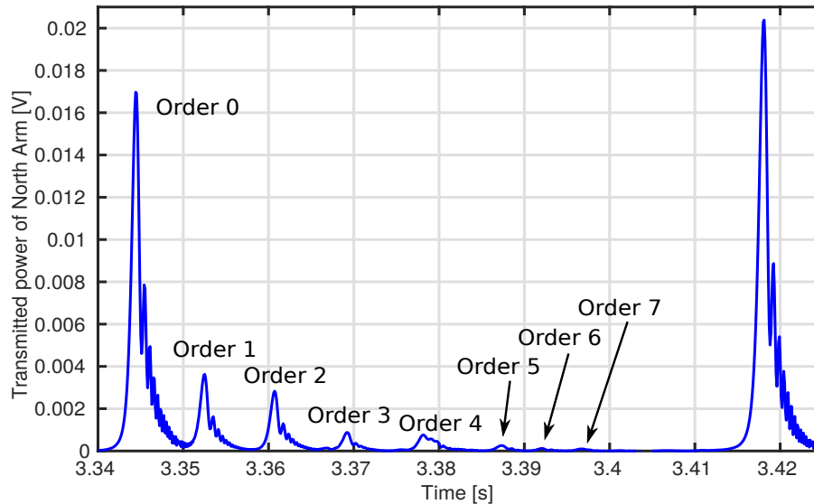
FIGURE 4.9: Transmitted power during a scan of the North Arm Cavity length. The two highest peaks correspond to the fundamental mode, meanwhile the smaller peaks are the HOMs. The closer peak to the TEM 00 correspond to the first HOM, the second closer to the second HOM and so on. HOMs can be seen up to the seventh order, even if the two last are very small.
