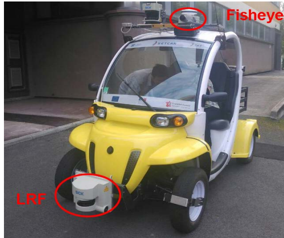
Figure 3-15: The configuration of the used experimental platform
