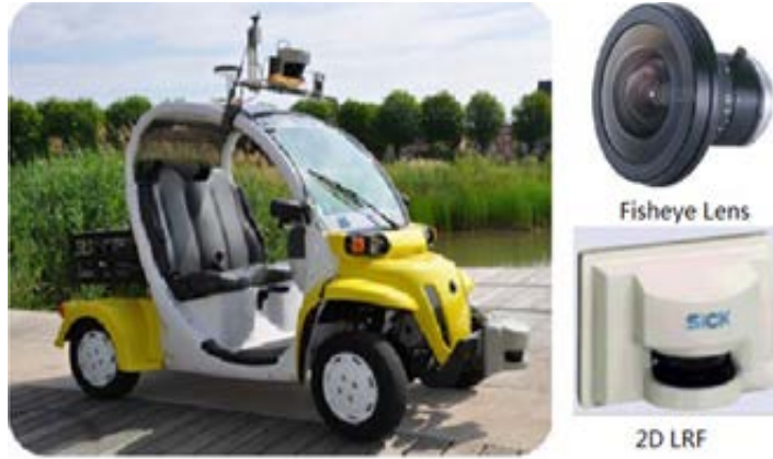
Figure 2-1: The experimental platform. The fisheye camera is on the top bracket and the LRF is fixed in front of the vehicle
