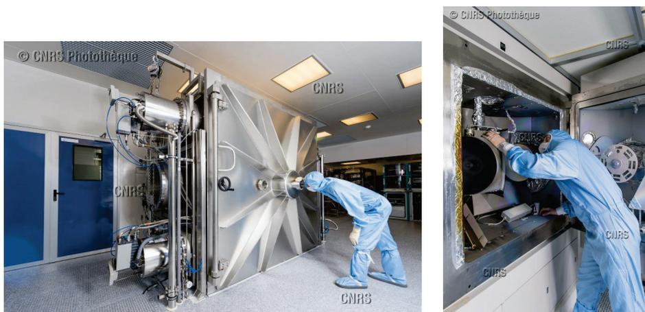
Figure 1.4 – Photos of the two coating chambers at the LMA, the Grand Coater on the left and the Spector on the right [Fresillon, 2016].
