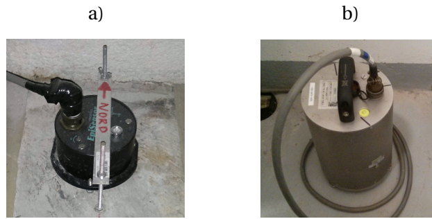
Figure 3.5 – Episensor FBA EST tri-axial accelerometer (a) and CGM40 tri-axial velocimeter (b) used for the comparison.
