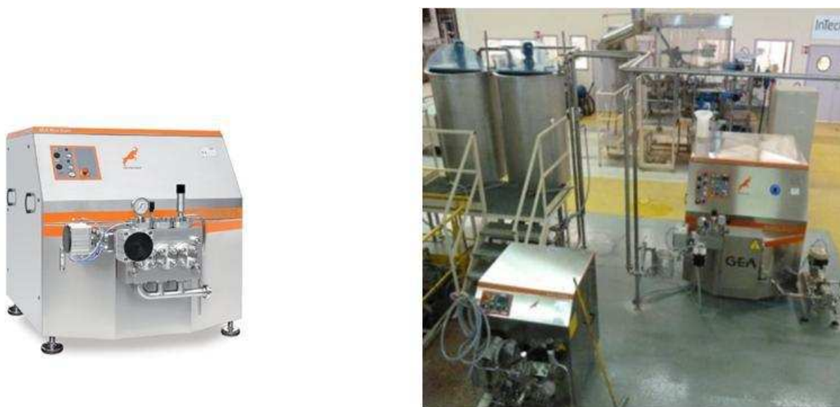
Figure 26: GEA Ariete homogenizer and picture of the NaMiCell pilot plant (CTP)
