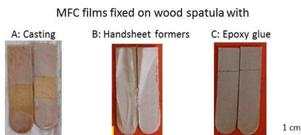
Figure 78: Illustration of MFC film fixed on wood spatula with A : casting, B : handsheet formers, C : epoxy glue
