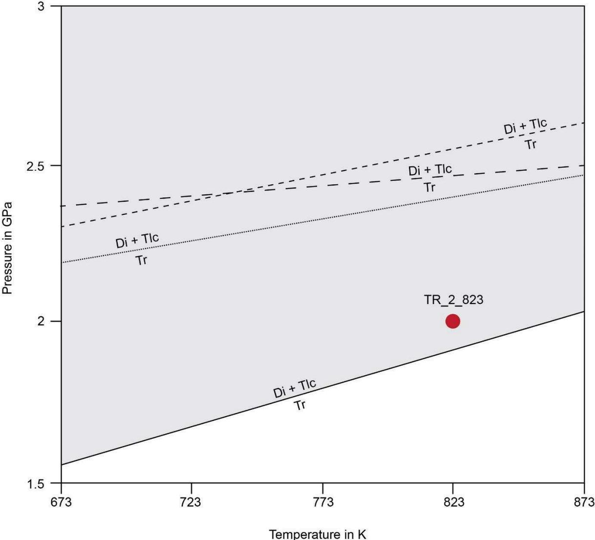
Figure 80: P-T conditons of the hydrostatic experiment TR\_2\_823.
