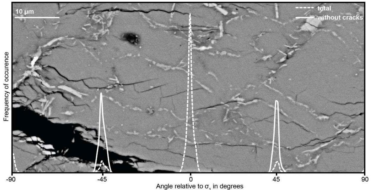
Figure 66: BSE image of the sample NG\_3\_1225 shows an area selected for a structure distribution plot using the software ImageJ. Both groups of Cz-bands are oriented either  $45$  or  $-45^\circ$  towards  $\sigma_1$ . The dashed line shows the measurement of all detected structures, cracks included, and the solid white line only the distribution of the Cz-bands with respect to  $\sigma_1$ .
