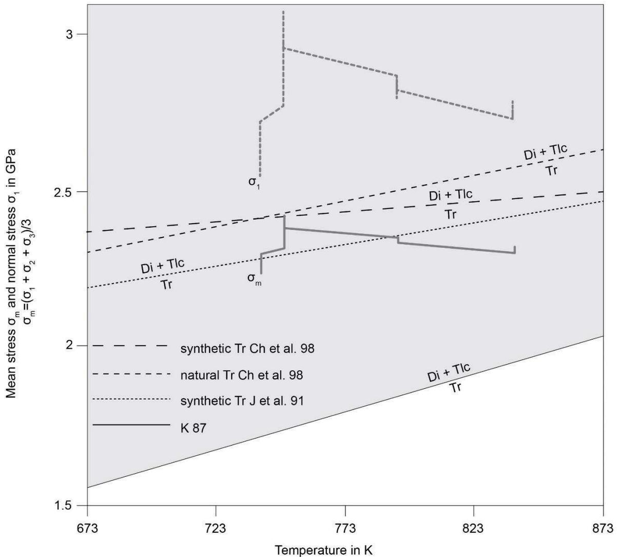
Figure 93: Mean normal and principal normal stress vs. temperature plot showing the influence of both stresses on the phase stability. Due to the increase in  $\sigma_1$  the sample could enter the stability field of diopside and talc, although the confining pressure  $P_c$  ( $\approx 2$  GPa) lies beyond this phase boundary (except for the phase diagram from Kirby, 1987).
