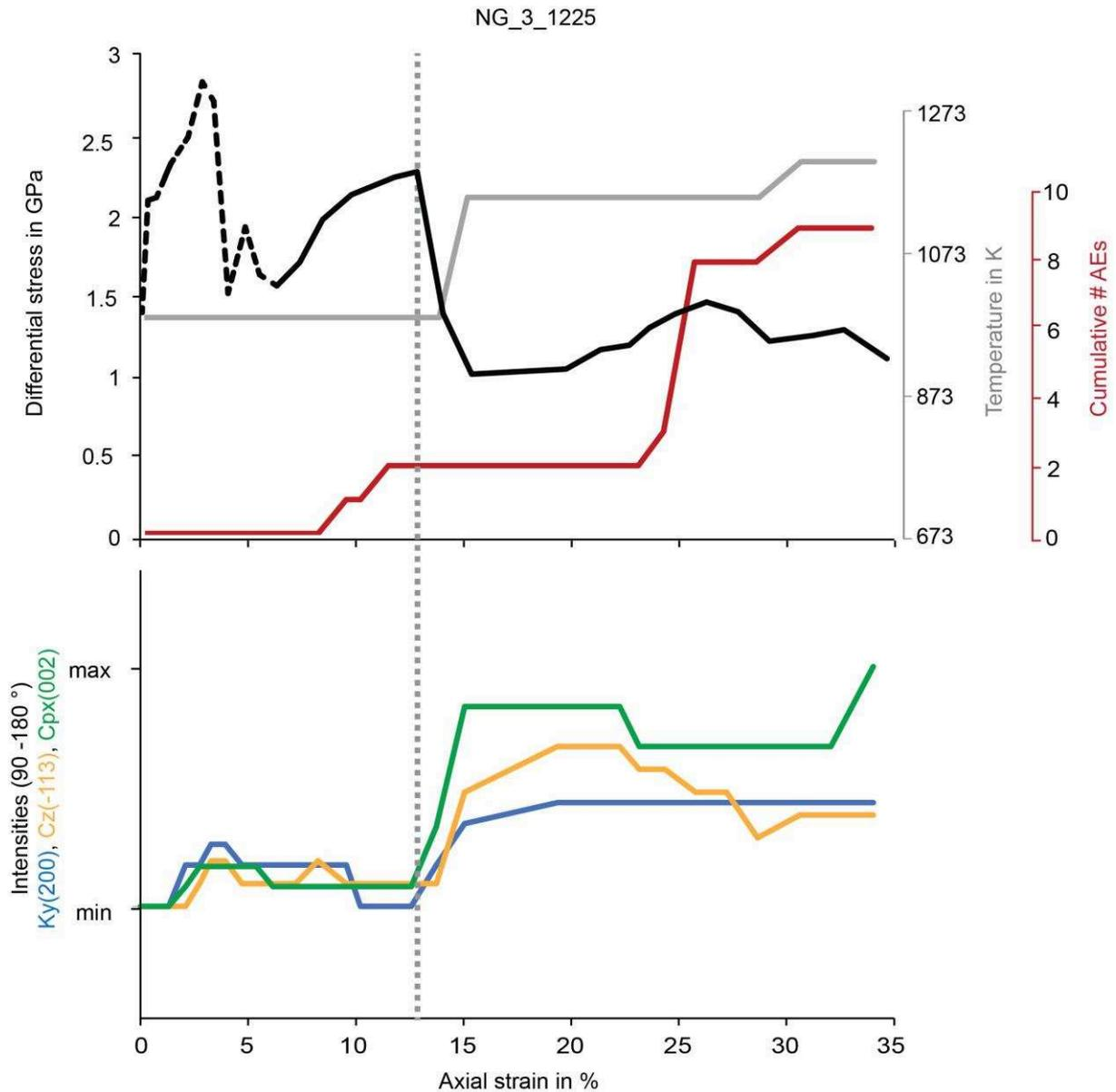
Figure 61: Mechanical data and XRD observation during deformation of the sample NG\_3\_1225. Differential stress (black), temperature (grey), and cumulative number of AEs (red) over axial strain in %. The lower plot shows the textural evolution of the intensities of Ky (200), Cz (-113), and Cpx (002). In this run the onset of AEs does not correlate with the stress drop at 12 % axial strain.
