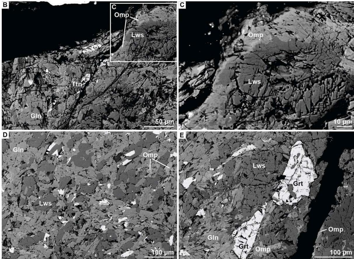
Figure 46: Four different BSE images showing higher magnification images of sample BSd\_3\_823. B) Corner of the sample exhibits fractures with omphacite (Omp) along its borders. C) Closer magnification of an area marked in B). D) Region in the sample unaffected by fracturing. Much less Omp can be found in these areas compared to the vicinity of fractures. E) Dissected and displaced garnet crystal along a narrow fault.
