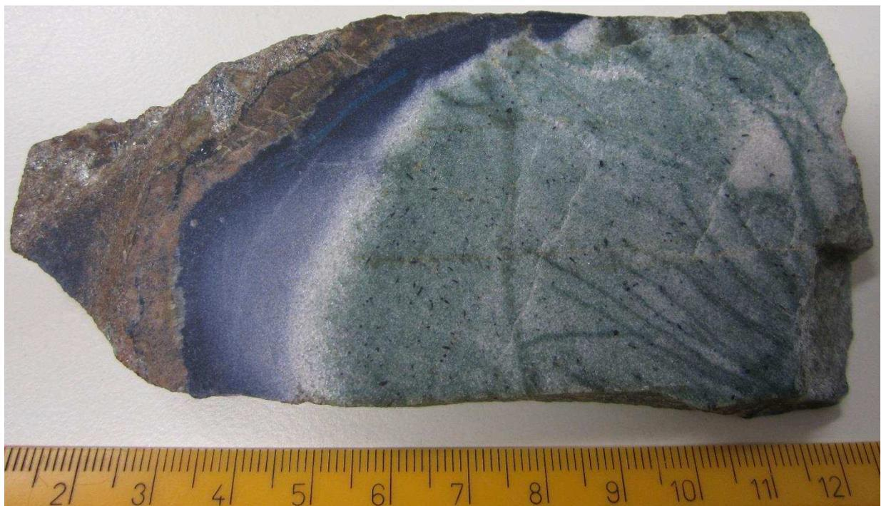
Figure 15: Handspecimen provided by Prof. Timm John. Only a small part from the blue layer, identified as blueschist, was taken for the production of the starting material.
