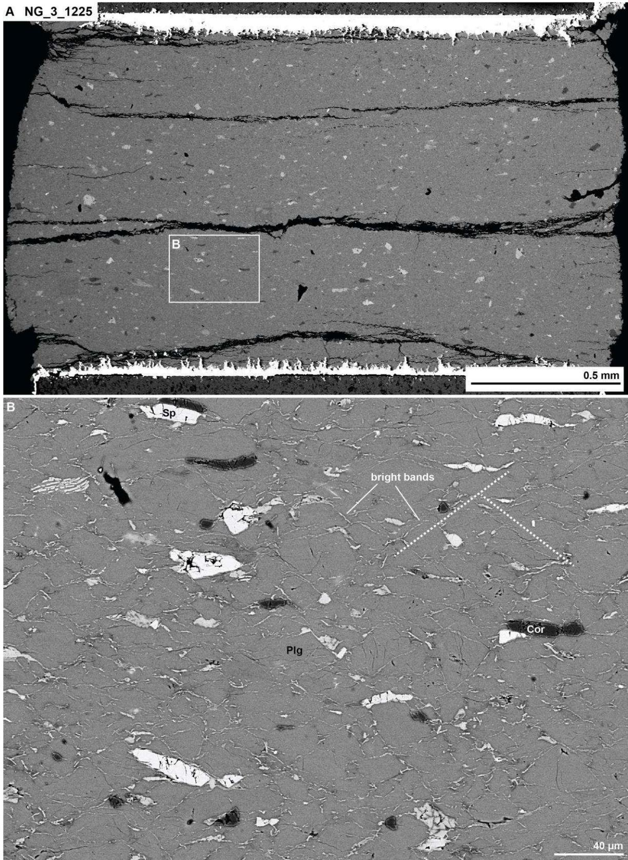
Figure 65: Sample NG\_3\_1225 after deformation. A) Many decompression cracks cut horizontally through the sample. B) The microstructure of this sample reveals two group of bands mostly composed of clinozoisite crystals. The bands of each group are all oriented more or less parallel to each other.
