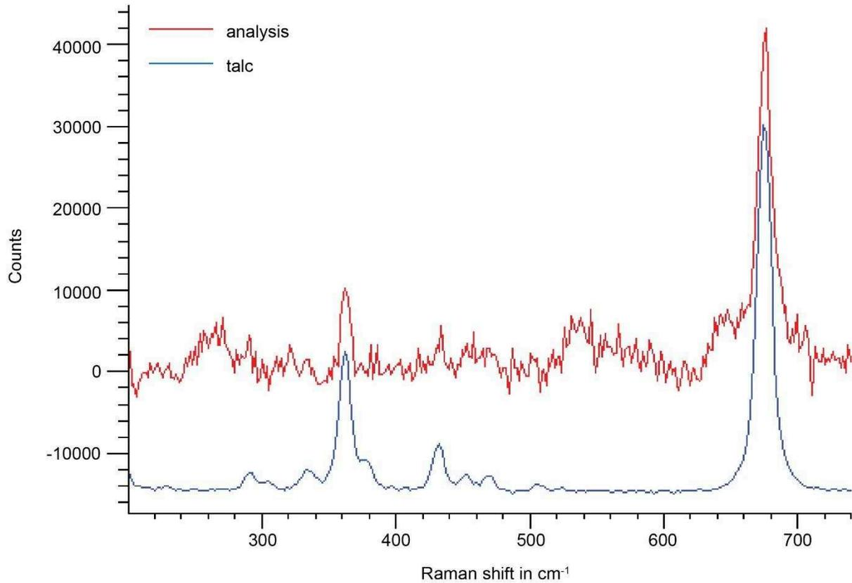
Figure 91: Raman analysis of the newly grown phase identified as talc in the tremolite experiment TR\_2\_838.
