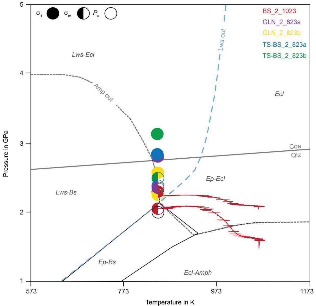
Figure 50: The powder deformation experiments were conducted under isothermal conditions except the run BS\_2\_1023 (red circles and curves), which was heated from 823 to 1023 K. Filled circles show the respective  $\sigma_1$  (based on axial load data) and half-filled circles the calculated  $\sigma_m$  for each run.
