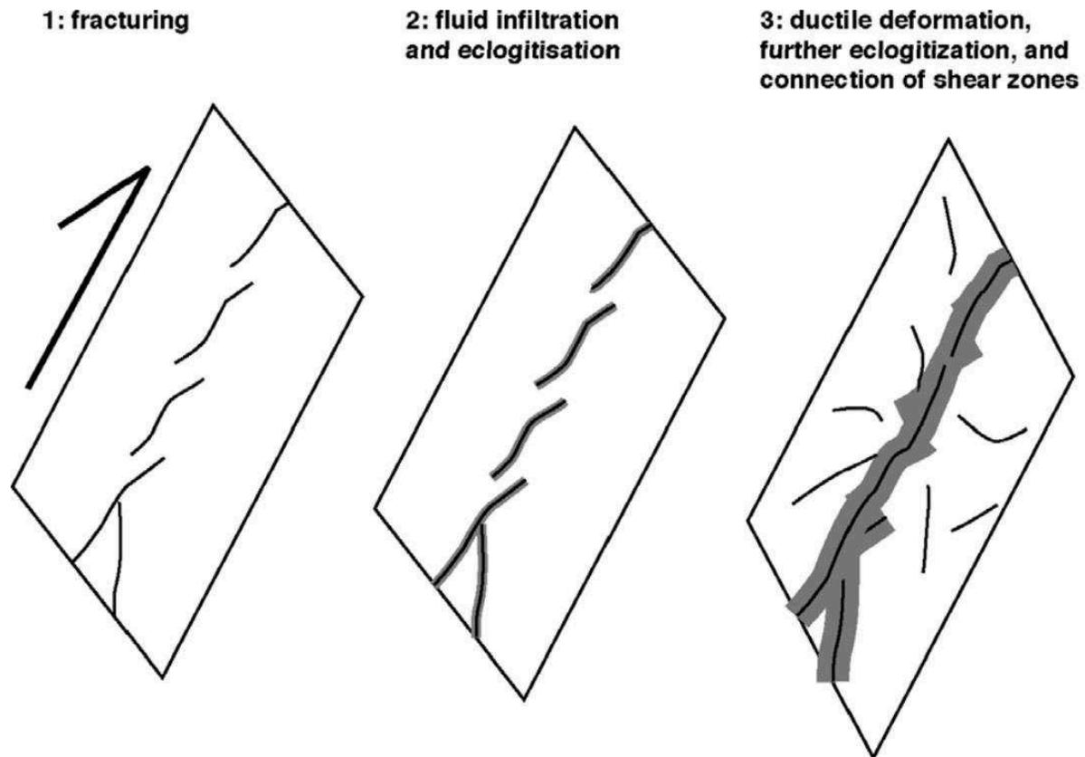
Figure 79: From Jolivet et al. (2005). Schematic drawing showing the evolution from brittle to ductile deformation due to the eclogitization of granulite.
