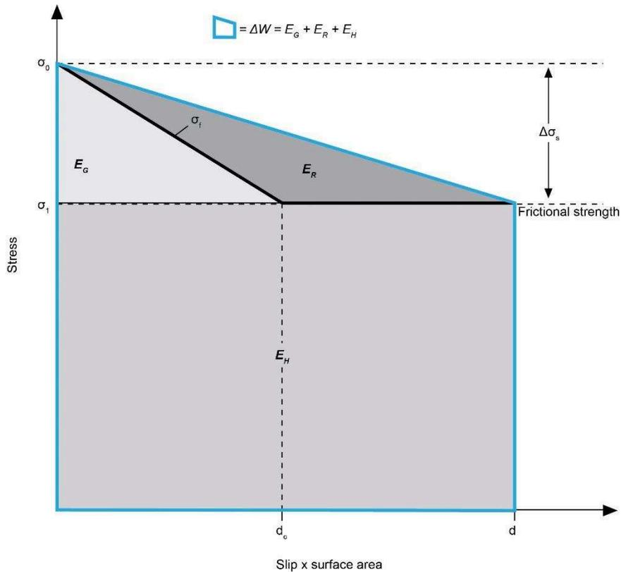
Figure 95: Schematic drawing of the slip weakening model demonstrating the expected energy partitioning released during an earthquake.
