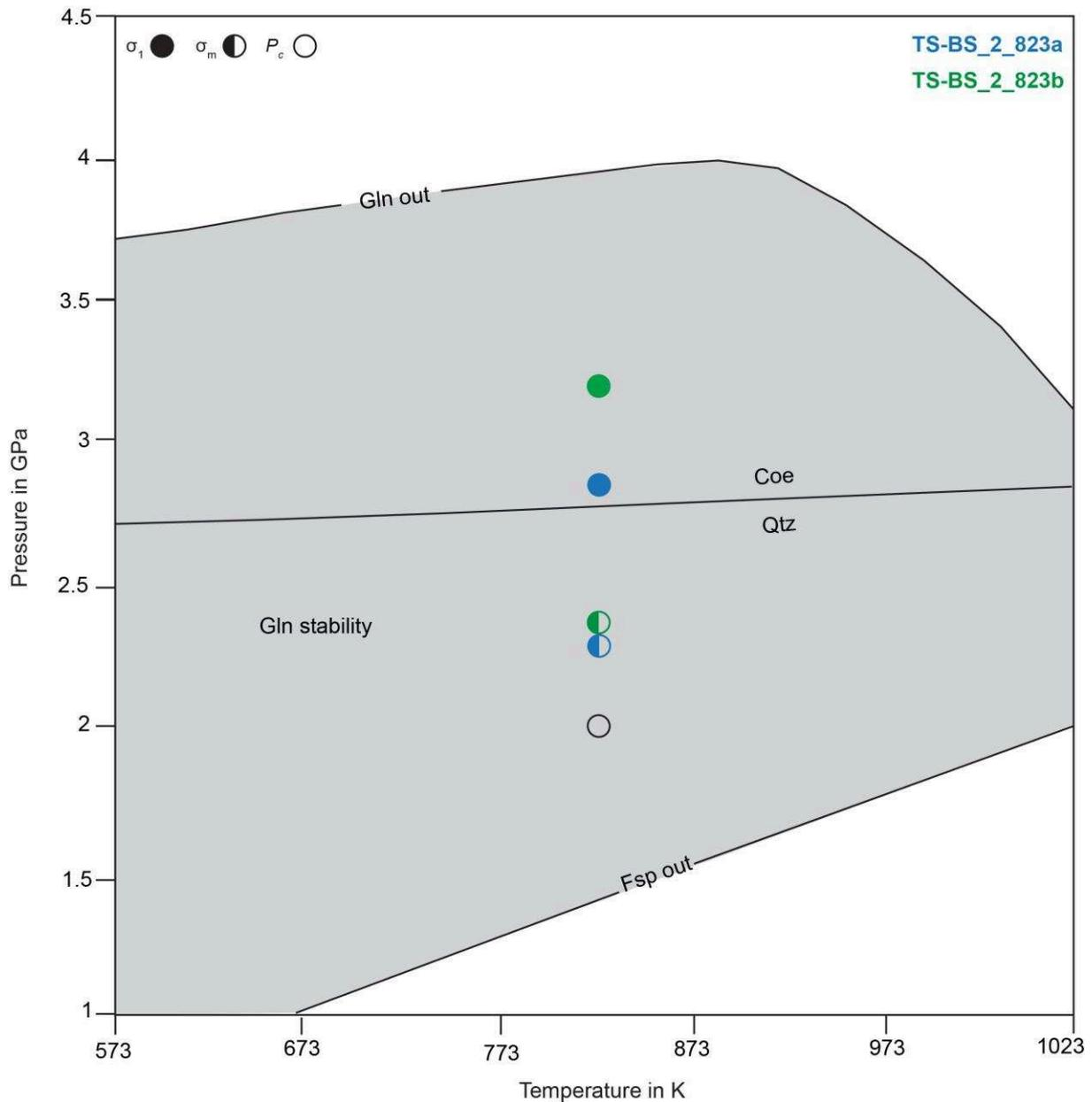
Figure 56: Griggs experiments on Tianshan blueschist powders (TS-B2\_823a in blue and TS-B2\_823b in green) superimposed on the P-T pseudosection of the bulk rock chemistry of the Tianshan blueschist (Klemd et al., 2015) calculated using Theriak Domino.
