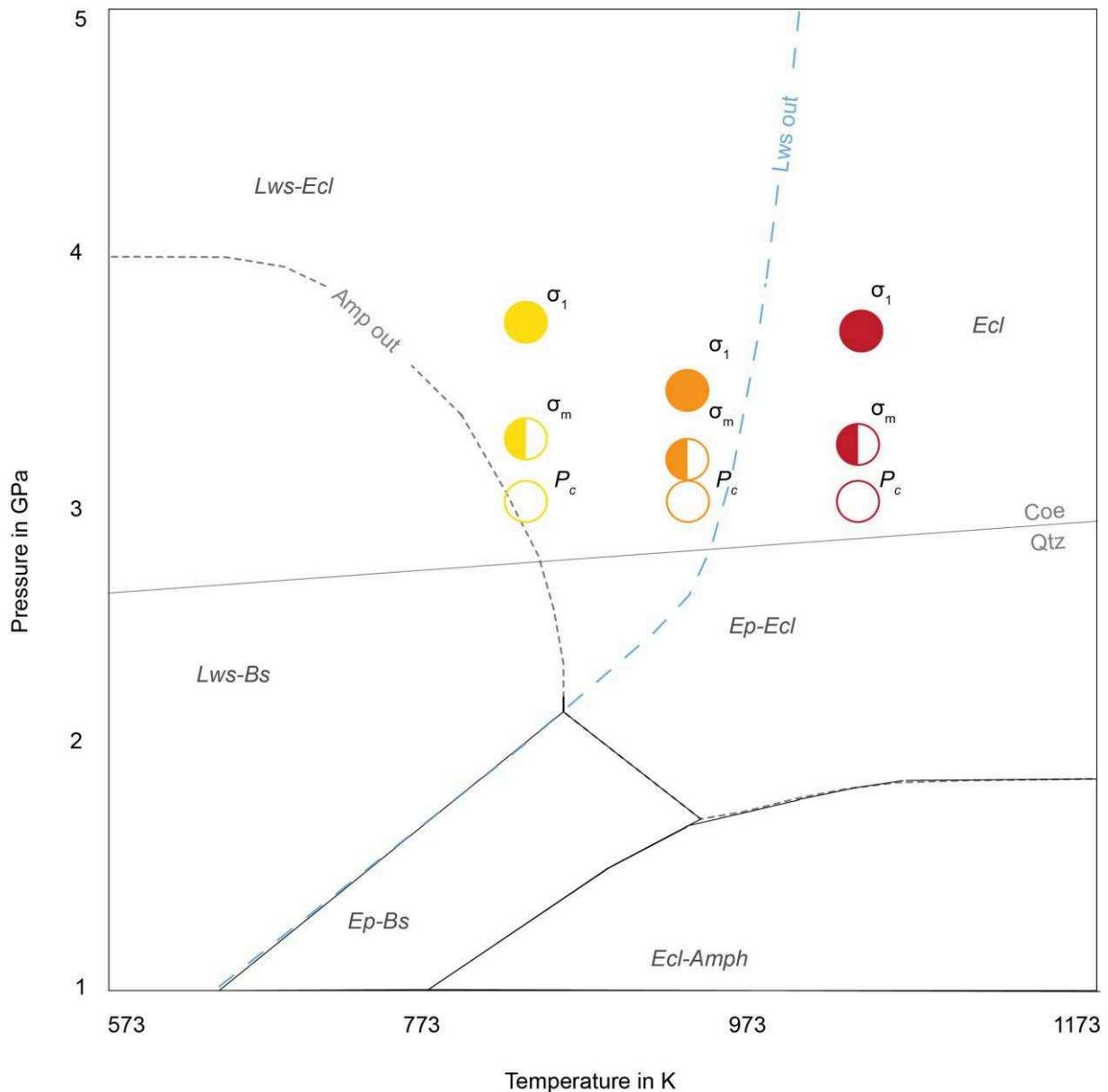
Figure 47: P-T pseudosection with superimposed  $P_c$ ,  $\sigma_m$ , and  $\sigma_1$  for the deformation experiments performed on the intact Corsican blueschist drill cores. Yellow colored circles represent the experiment conducted at 823 K, orange circles at 923 K, and red circles at 1023 K.
