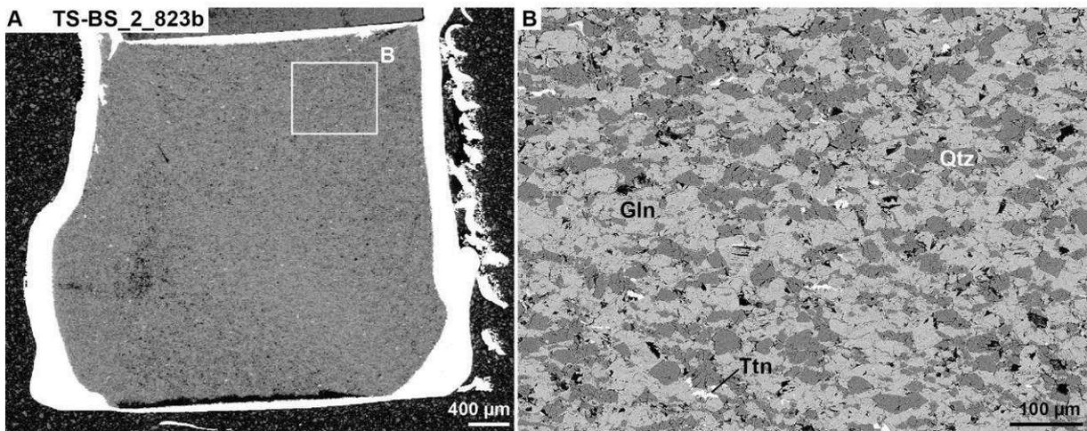
Figure 54: The microstructure of the sample TS-BE\_2\_823b shows no evidence for macro- or microscopic strain localization.
