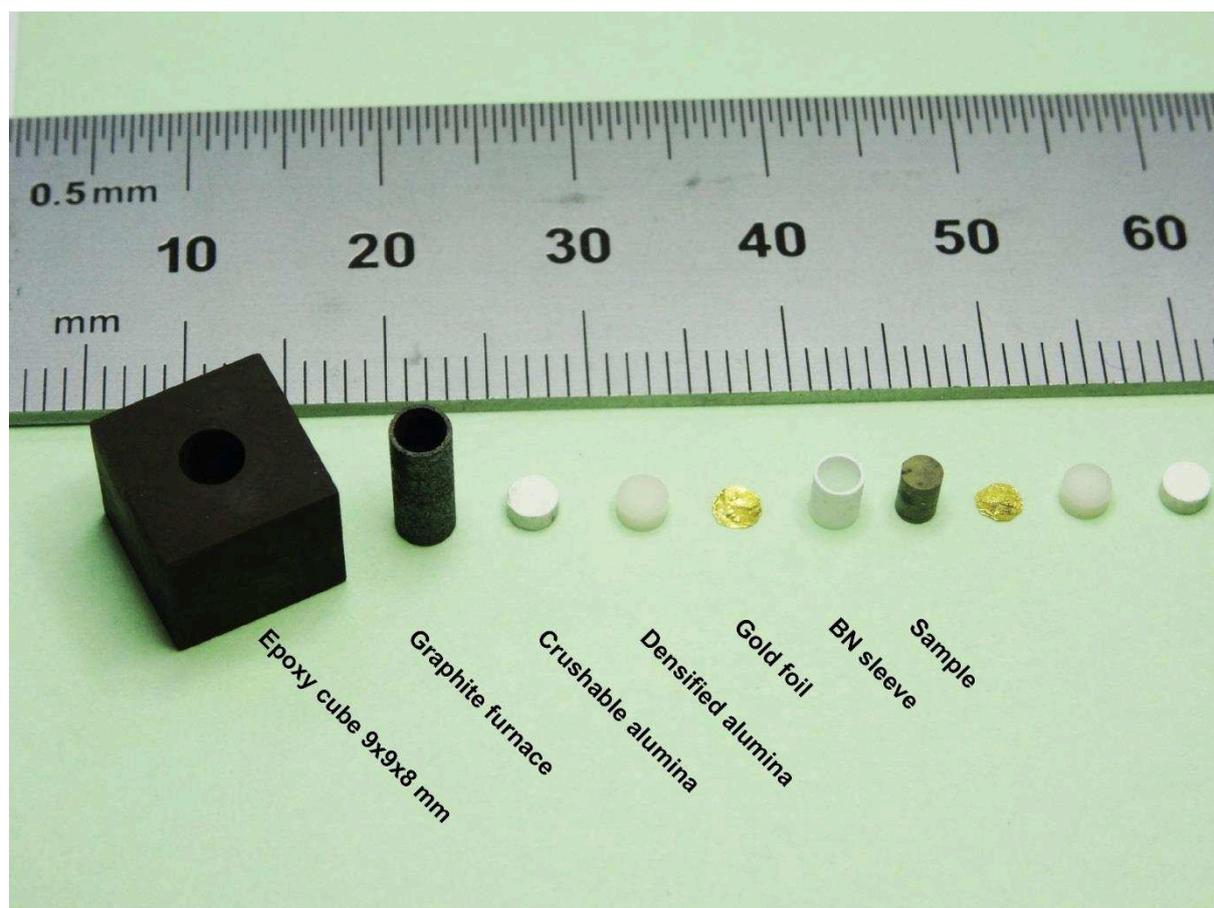
Figure 31: Sample assembly for the D-DIA deformation experiments.
