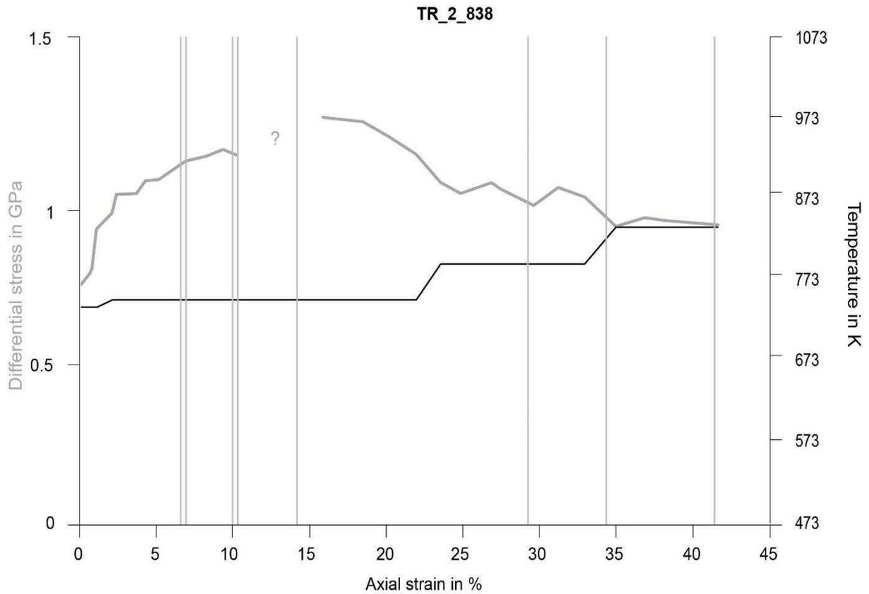
Figure 86: Differential stress (grey line) and temperature (black line) vs. axial strain in %. Due to an insufficient quality of the powder diffraction images it was not possible to calculate the differential stress on tremolite between around 11-16 % axial strain. This region is marked with a question mark. The grey bars highlight the occurrence of the recorded AEs during deformation.
