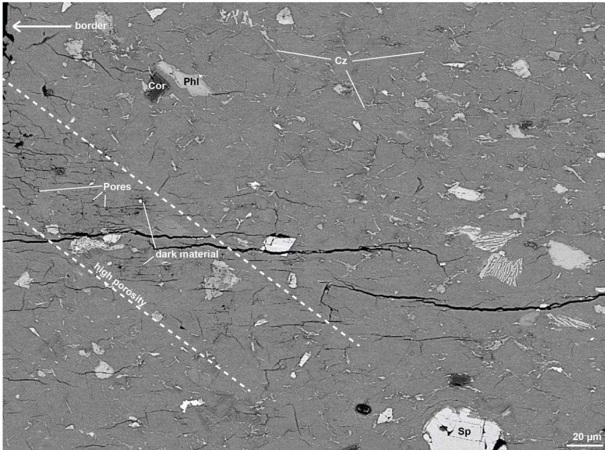
Figure 69: The sample NG\_3\_1225 is almost entirely covered by these bright Cz-bands, but some in which these bands are missing show an increase in porosity. This zone forms a band in an angle of about  $45^\circ$  towards  $\sigma_1$
