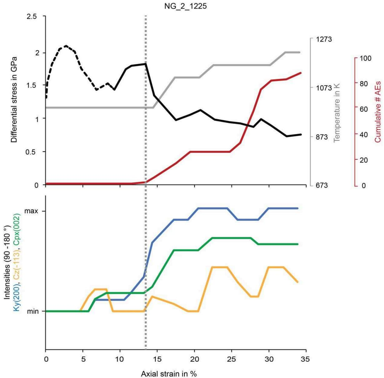
Figure 60: Mechanical data and XRD observation during deformation of the sample NG\_2\_1225. Differential stress (black), temperature (grey), and cumulative number of AEs (red) over axial strain in %. The lower plot shows the textural evolution of the intensities of Ky (200), Cz (-113), and Cpx (002). The stress drop at around 12 % axial strain coincides with the onset of AEs.
