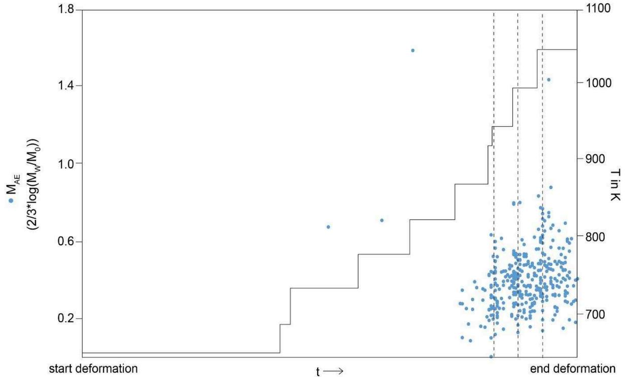
Figure 83: Magnitude of AE ( $M_{AE}$ ; each blue spot corresponds to one recorded event) and temperature (black line) over time plot presenting the energy of each event and their occurrence during deformation of the sample GLS\_3\_1043.
