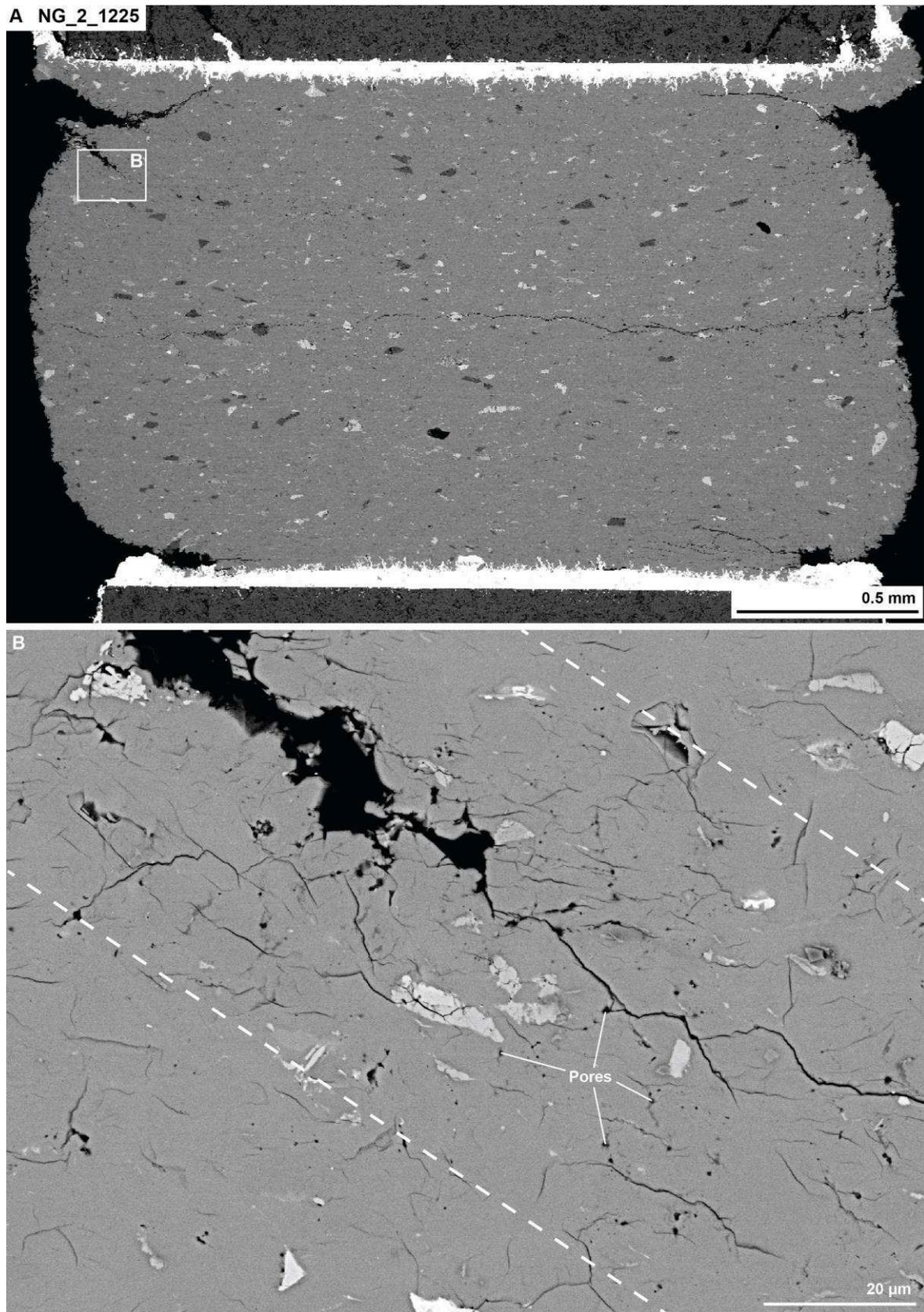
Figure 62: BSE images of the D-DIA sample NG\_2\_1225. A) Overview image demonstrating the location of the higher magnification image shown in B. B) Zone with higher porosity within the vicinity of a small fracture.
