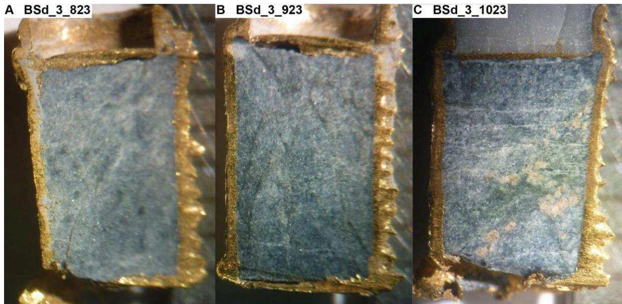
Figure 44: Optical microscopy images of the drill core samples after deformation. A)  $P_c = 3$  GPa,  $T = 823$  K; B)  $P_c = 3$  GPa,  $T = 923$  K; C)  $P_c = 3$  GPa,  $T = 1023$  K. The strain rate was constant during each experimental run with around  $2 \cdot 10^{-5} \text{ s}^{-1}$ .
