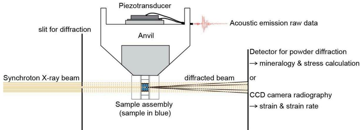
Figure 30: Schematic drawing of the experimental setup for the D-DIA experiments. For the sake of clarity only the upper vertical anvil is shown.
