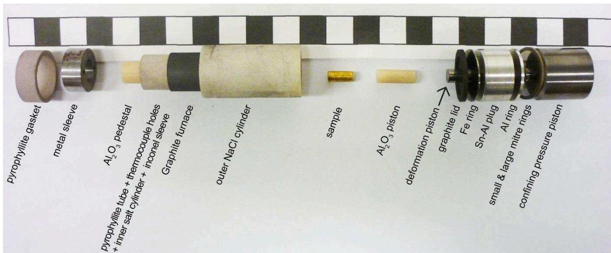
Figure 28: Image of the sample assembly where a combined deformation piston was used for the experiments. The  $\text{Al}_2\text{O}_3$  was left out for powder experiments conducted under 823 K.
