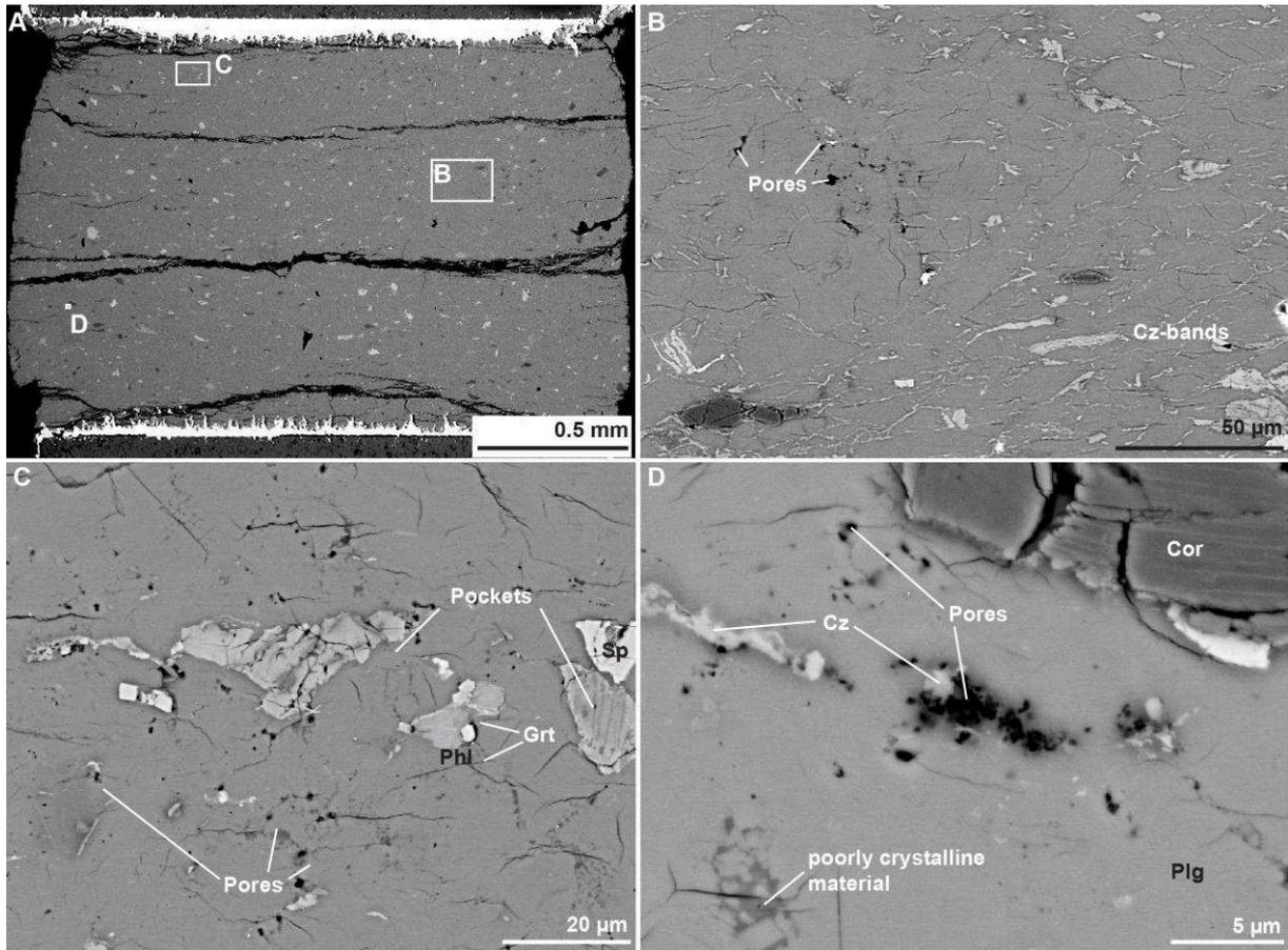
Figure 70: BSE images of the sample NG\_3\_1225 exhibiting areas of high porosity in which Cz-bands are absent (A). B) Many pores appear together with dark (relative to plagioclase in BSE mode) patches. C) Compared to Plg grains from the starting material, very small Plg crystals can be found within dark patches of poorly crystalline material. D) Idiomorphically shaped Grt crystal floating within a poorly crystalline material.
