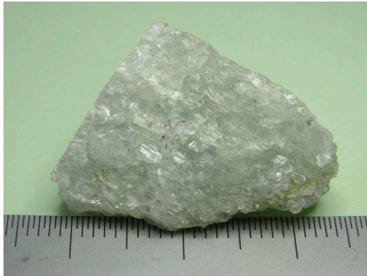
Figure 19: The tremolitite sample used for the experiments was provided by Prof. Pamela Burnley. The sample consists almost purely of tremolite (Kirby, 1987).
