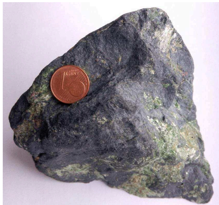
Figure 20: Blueschist sample from Syros, Greece. This sample was provided L. Labrousse The bluish parts of the hand specimen are made of glaucophane. The greenish areas mostly consists of chlorite.
