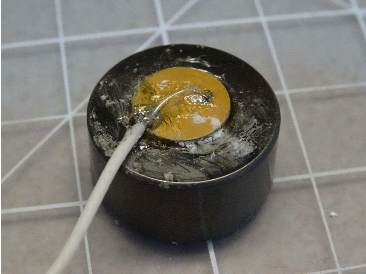
Figure 39: Custom-made acoustic emission sensor used for the deformation experiments at the APS Chicago.
