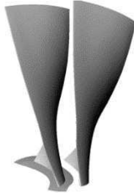
Figure 4.21: Typical shape of a turbomachine fan blade.
