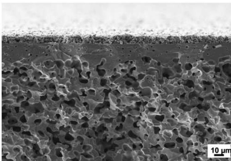
Figure 1.17: Cross section of an asymmetric membrane assembly consisting of porous support, dense membrane layer, and porous surface activation layer made from  $Ba_{0.5}Sr_{0.5}Co_{0.8}Fe_{0.2}O_{3-\delta}$  [2]
