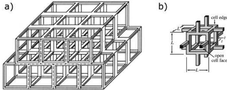
Figure 1.4: Idealized unit cell in an open cell foam
