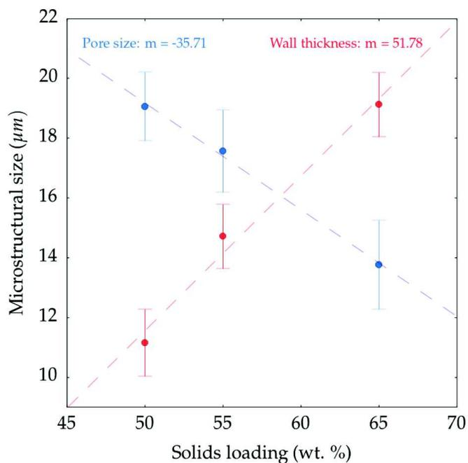
Figure 3.4: Wall thickness and pore size dependency on solids loading. Samples were frozen at 2 °C/min and both microstructural dimensions obtained by image analysis.  $m$  corresponds to the slope of the trendline.
