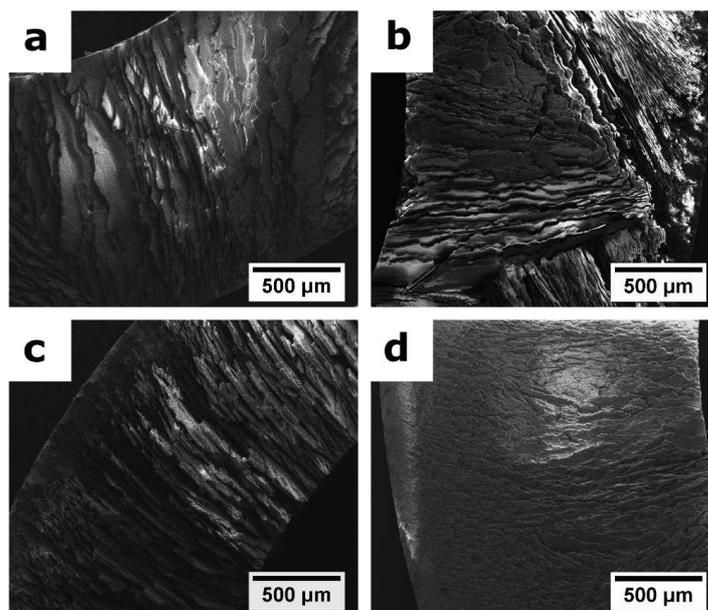
Figure 6.3: Detail of the radial porosity of ice-templated tubes sections reported in Table 6.1. a) 50 wt.% solids loading and freezing temperature  $-30^{\circ}\text{C}$ , b) 50 wt.% solids loading and freezing temperature  $-80^{\circ}\text{C}$ , c) 65 wt.% solids loading and freezing temperature  $-30^{\circ}\text{C}$ , and d) 65 wt.% solids loading and freezing temperature  $-80^{\circ}\text{C}$ . In all cases the volume of slurry used was 20ml.
