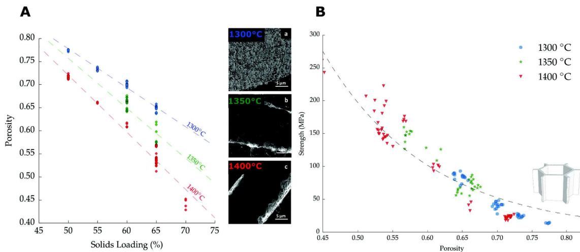
Figure 4.9: (A) Effect of solid loading and sintering temperature on % porosity and evolution of wall densification. (B) Relation between compressive strength and total pore volume for ice-templated samples frozen at 2 °C/min, with a pore size in the range of 10-20  $\mu\text{m}$ , and sintered at different temperatures (1300-1400°C). Dashed line represents the honeycomb out-of-plane model, Eq. 4.3.
