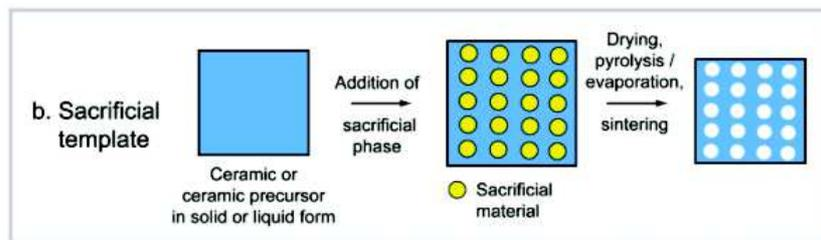
Figure 1.7: Scheme of the steps involved to obtain porous ceramics by the sacrificial template method [32]
