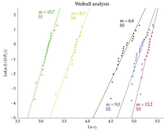
Figure 4.14: Weibull strength distributions of groups described in Table 4.2. The solid line represents the OLS fit to the data.
