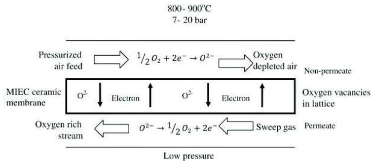
Figure 1.13: Different steps involved in oxygen transport during oxygen permeation [47]
