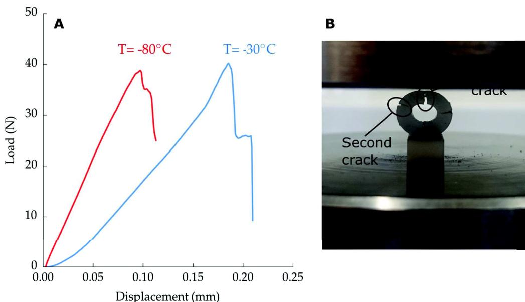
Figure 6.6: A) Representative load-displacement curves of two rings obtained from tubes with a 65% solids loading and frozen at  $-80^{\circ}\text{C}$  (red) and  $-30^{\circ}\text{C}$  (blue). B) Detail of the characteristic fracture in a O-ring test with the two types of cracks highlighted.
