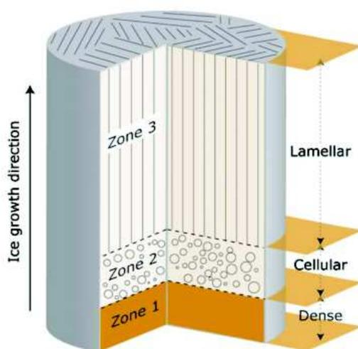
Figure 1.11: Typical porosity microstructure of an ice-templated samples showing the three distinctive zones [40]
