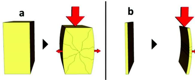
Figure 4.7: Representation of the different failure mode of the walls. a) Brittle fracture observed at low pore volume and b) Buckling fracture observed at high pore volume. Image extracted from [83].
