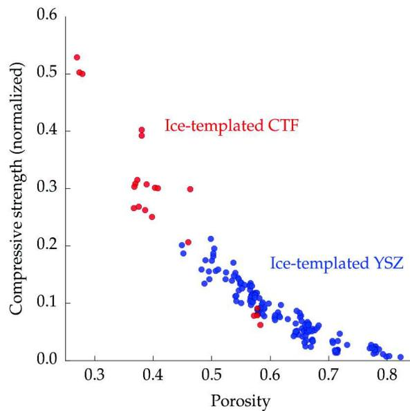
Figure 4.8: Compressive strength dependence on porosity for ice-templated samples frozen at  $2^\circ\text{C}/\text{min}$  in YSZ (blue) and CTF (red). The strength data was normalized by the flexural strength of the respective bulk material
