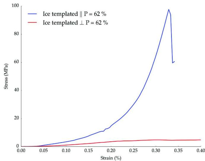
Figure 4.11: Representative stress-strain curves for two ice-templated specimens loaded parallel (blue) and perpendicular (red) to the pores. In both cases freezing temperature was  $2^{\circ}\text{C}/\text{min}$ . The solids loading, and hence porosity, is the same in both cases highlighting the high anisotropic behavior.
