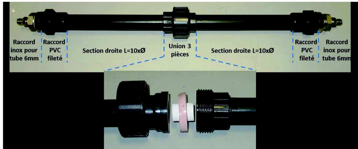
Figure 2.9: Set-up used to measure the pressure drop
