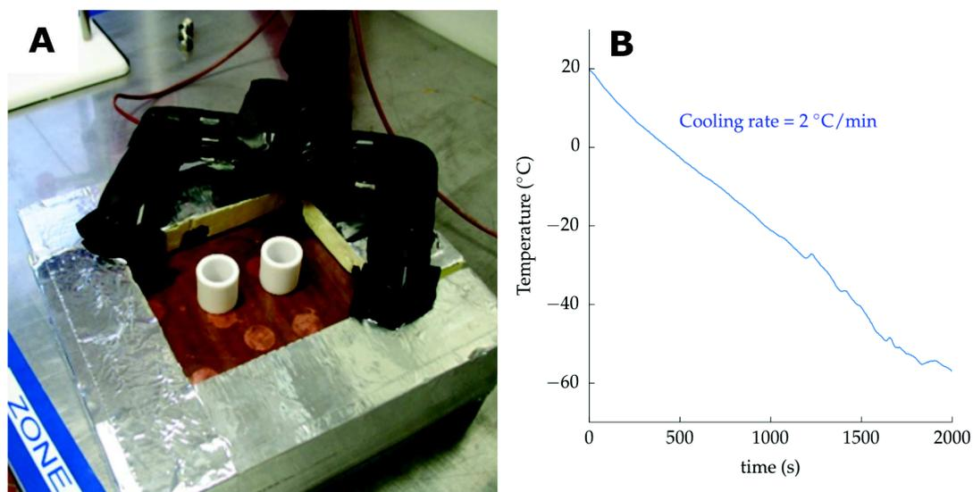
Figure 2.1: A) Freezing set-up used to achieve the cooling rate of  $2\text{ }^{\circ}\text{C}/\text{min}$ . B) Evolution of temperature with time for the set-up shown in a).
