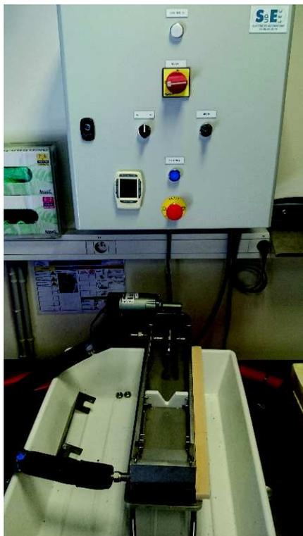
Figure 2.3: Set-up developed to freeze under rotation and produce ice-templated tubes.
