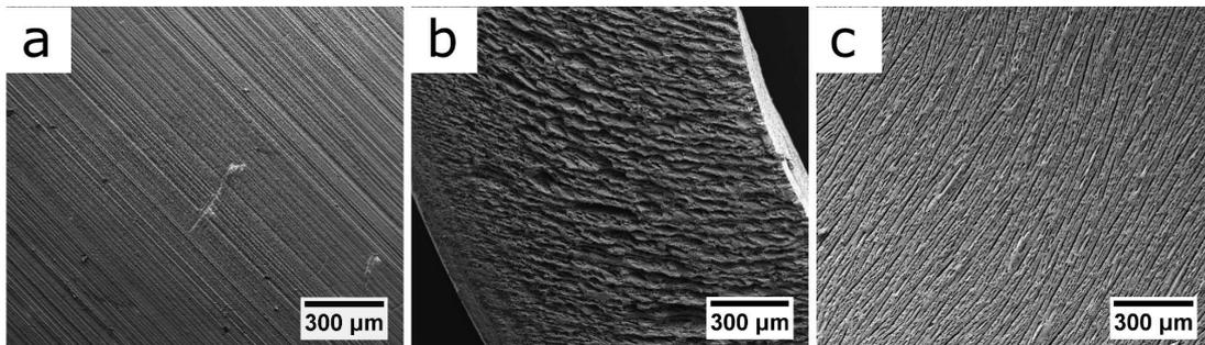
Figure 6.2: SEM micrographs of different locations of an ice-templated tube with a 65 wt.% solids loading, frozen at  $-30^{\circ}\text{C}$ , and 20 ml. A) Top view of the external layer B) Cross section of the tube and C) Top view of the inner surface.
