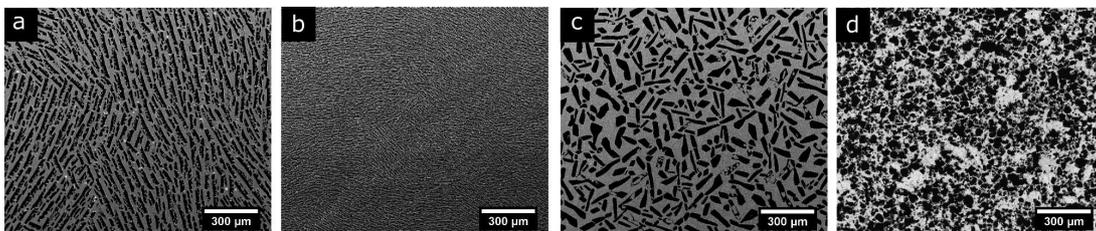
Figure 4.1: Micrographs of ice-templated samples a) frozen at  $2^\circ\text{C}/\text{min}$ , b) frozen at  $25^\circ\text{C}/\text{min}$ , c) frozen at  $2^\circ\text{C}/\text{min}$  with zirconium acetate (ZRA), and d) made by pore formers. In all cases the sintering temperature was  $1400^\circ\text{C}$  and the total pore volume was around 51%.
