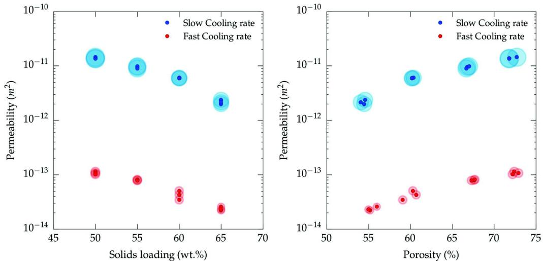
Figure 5.5: Effect of solids loading and freezing rate on permeability. Experimental and morphological parameters are specified in Table 5.1. Marker size is proportional to pore size.
