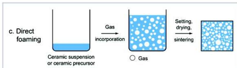
Figure 1.8: Schematic of a direct foaming technique [32]
