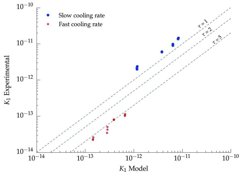
Figure 5.10: Comparison between the experimental permeability data and the values predicted by the capillary model
