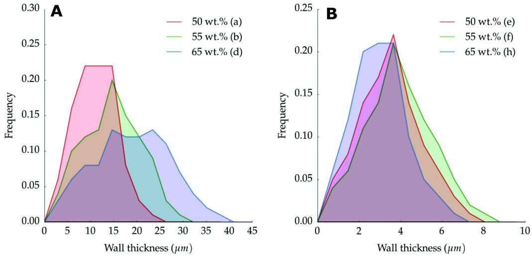
Figure 3.3: Pore size distribution obtained by image analysis of ice templated samples frozen at A) 2 °C/min B) 25 °C/min.
