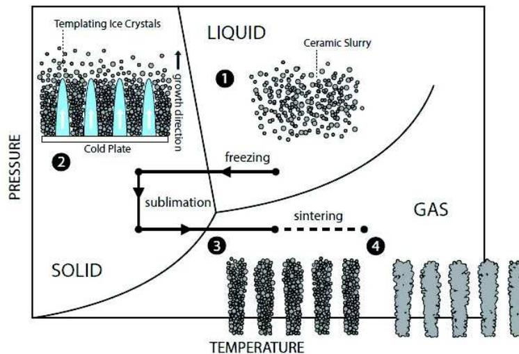
Figure 1.9: Processing steps of ice-templating [36]
