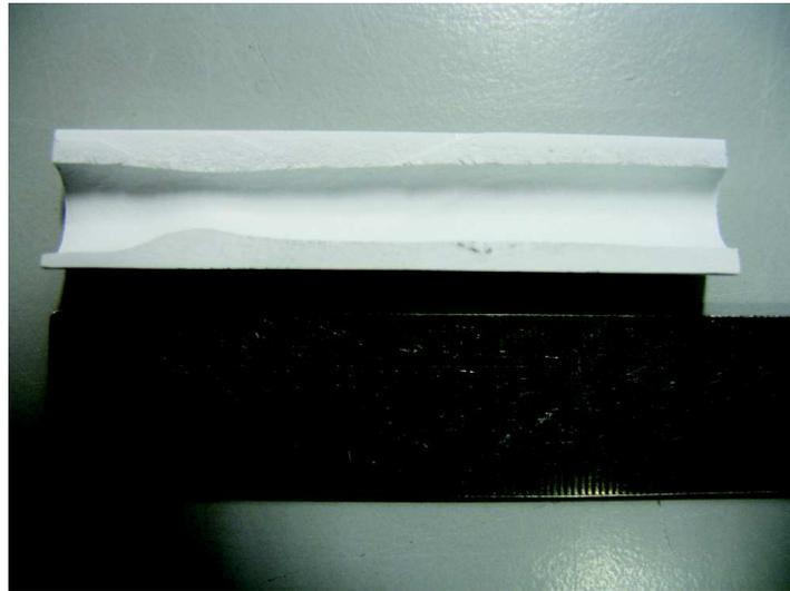
Figure 6.10: Detail of the thickness inhomogeneity in a four-point bending sample.
