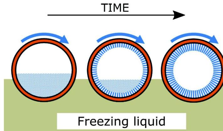
Figure 6.1: Schematic of the rotational freezing process.
