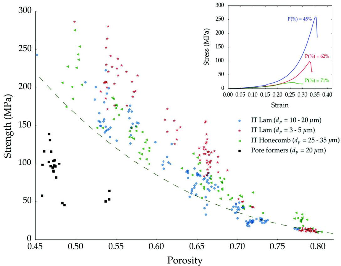
Figure 4.6: Compressive strength dependence on porosity in ice templated for samples frozen at  $2^\circ\text{C}/\text{min}$  (blue),  $25^\circ\text{C}/\text{min}$  (red), and with a honeycomb morphology (green). Isotropic samples made in this work by sacrificial method are also represented (black). The dashed line corresponds to the Honeycomb out-of-plane model shown in Eq. 4.3.
