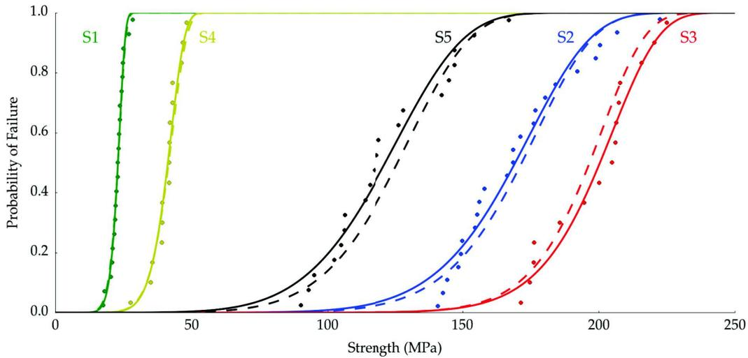
Figure 4.15: Probability of failure prediction based on the parameters  $\sigma_0$  and  $m$  shown in Table 4.2. The dotted lines are based on the OLS fitted parameters and the solid lines use parameters from the nonlinear Bayesian fit.
