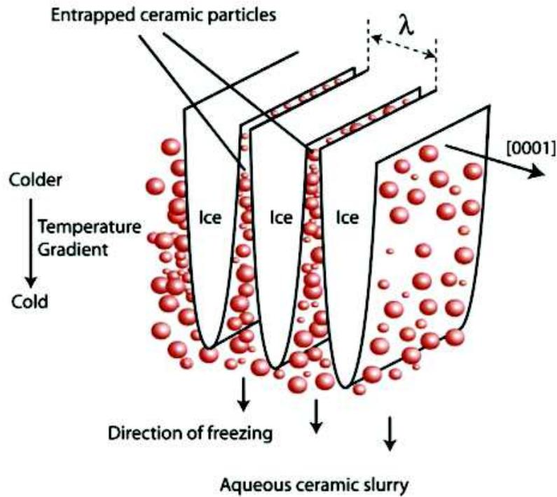
Figure 2: Schematic of the ice-templating process [6].
