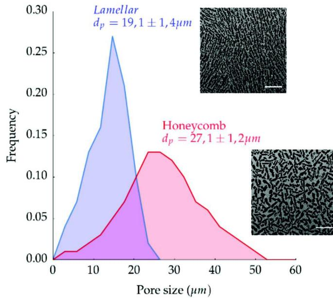
Figure 3.5: Pore size distribution of ice templated structures with ZRA (honeycomb) and without (lamellar). Solids loading used was 65 wt.% and freezing rate 2  $^{\circ}\text{C}/\text{min}$  in both cases. Scale bar = 300  $\mu\text{m}$
