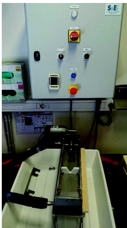
Figure 2.3: Set-up developed to freeze under rotation and produce ice-templated tubes.
