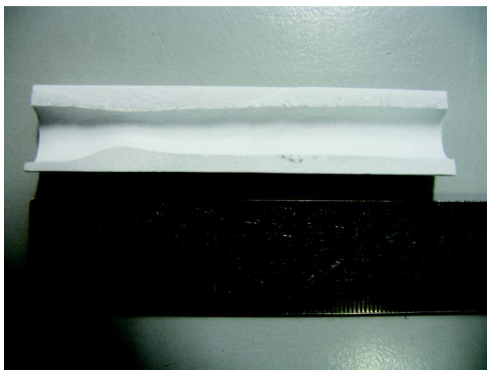
Figure 6.10: Detail of the thickness inhomogeneity in a four-point bending sample.
