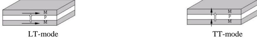
Figure 2.3 Illustration of the LT and TT modes for a trilayer ME composite
