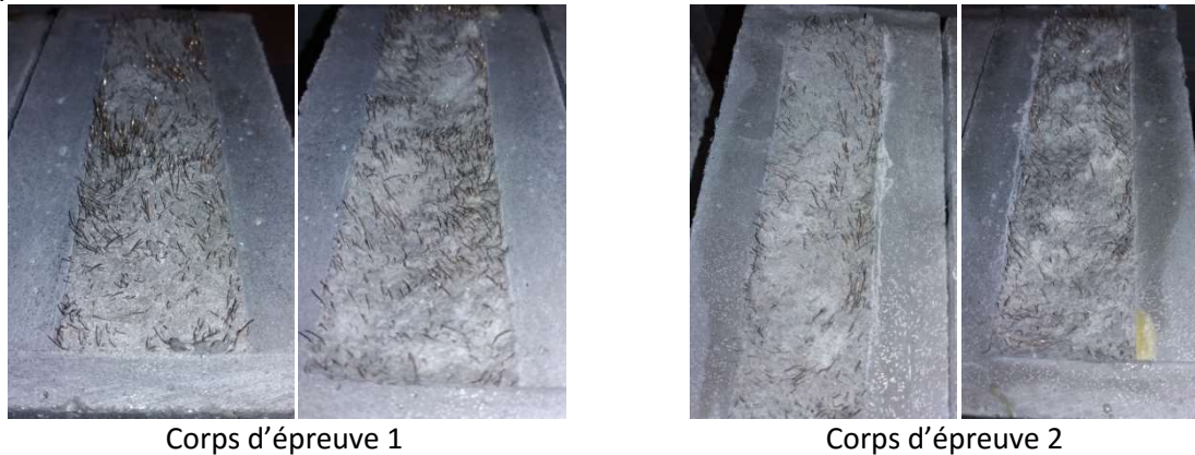
Figure 154: Aspect des surfaces de rupture BFUP B
