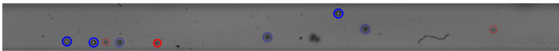
Fig. 5-2 Particle identification in the bidisperse suspension ( Re = 5.6 ). 8.7\text{-}\mu\text{m} and 5.3\text{-}\mu\text{m} particles are surrounded by blue and red circles, respectively, and the in-focus and out-of-focus particles by bold and thin circles, respectively.
