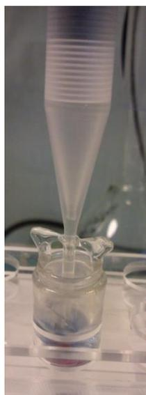
**Figure 76:** Clark-type H<sub>2</sub> microsensor immersed in a solution containing methyl viologen, sodium dithionite and 2-MeHydA. The blue/violet color is due to reduced methyl viologen.
