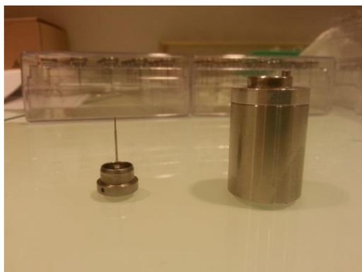
**Figure 83:** Loop (left) and device for crystal freezing inside the glove box (right). The cylindrical chamber is filled with liquid propane, frozen in liquid nitrogen and entered in the anaerobic chamber.
