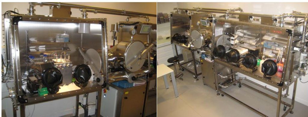
Figure 82: Pictures of glove boxes for protein crystallography. The chamber on the left side contains the Oryx Nano crystallization robot.
