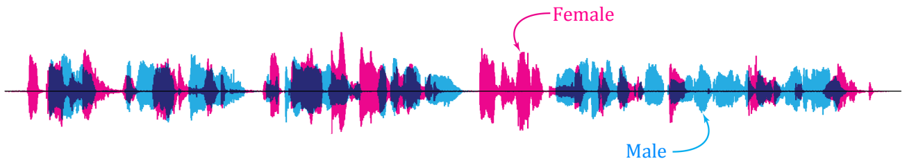
Figure 5 – Waveform of two voices, one male (light blue) and one female (magenta). On some time-windows the two voices overlap (dark blue parts) and on some other time-windows the two voices alternate without overlapping. This figure shows that solving this auditory scene implies to deal with both simultaneous and sequential mechanisms.
