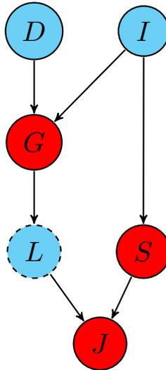
Figure 3.6: The Markov blanket for node  $L$
