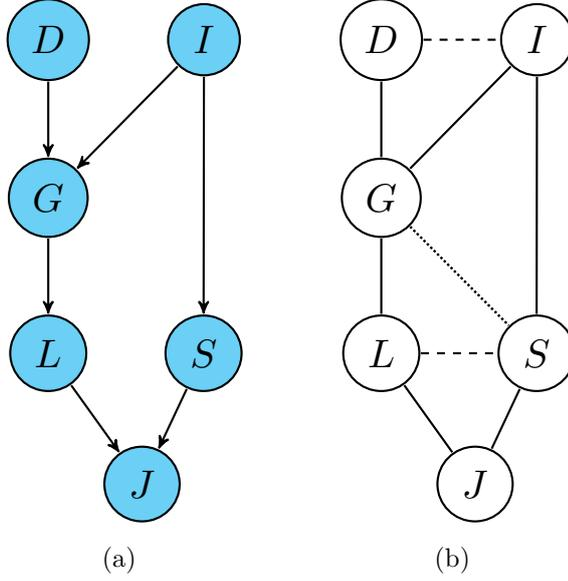
Figure 4.1: A DAG (a) and its corresponding moral then triangulated graph (b)
