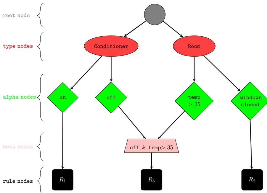
Figure 2.3: Rete network for air conditioner's Example 2.3.1
