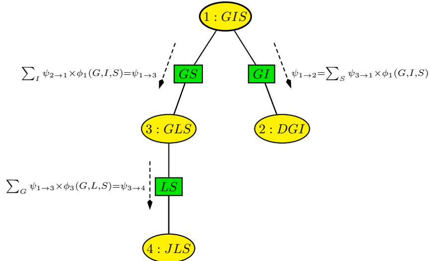
Figure 4.5: Message-passing during *distribution*
