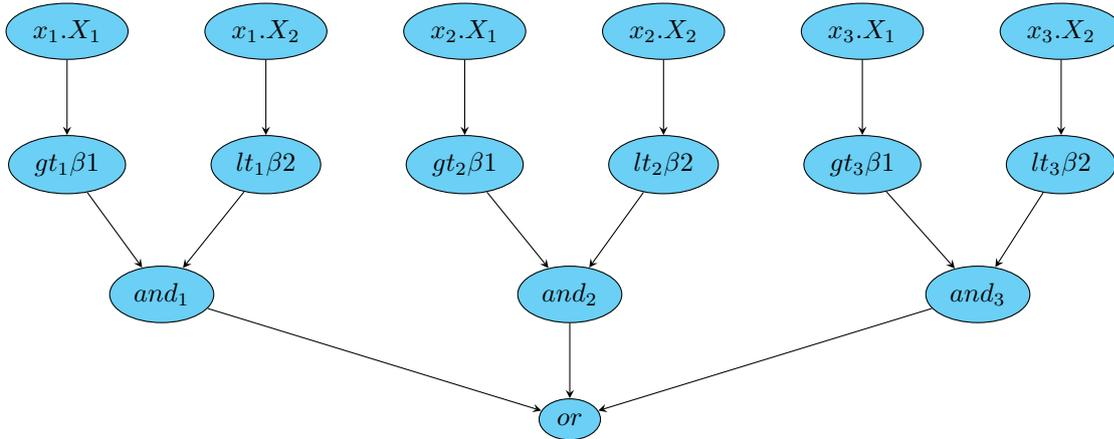
Figure 5.17: A runtime BN fragment obtained after compiling the existence condition in Rule 5.9
