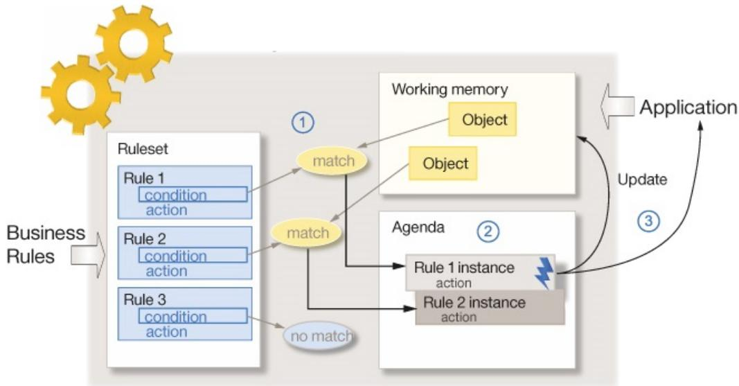
Figure 5.8: ODM rule engine in Rete mode
