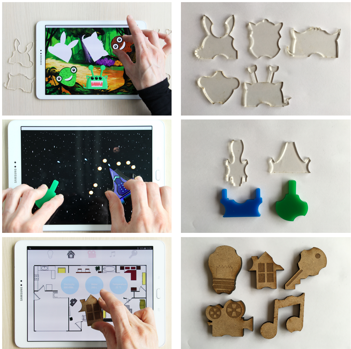
Figure 5.7: The three proof-of-concept token sets: toy characters (top), home automation (middle) and spaceship game (bottom).
