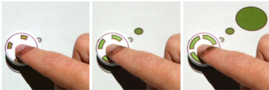
Figure 2.16: A Gecko token can sense pressure applied on top of it
