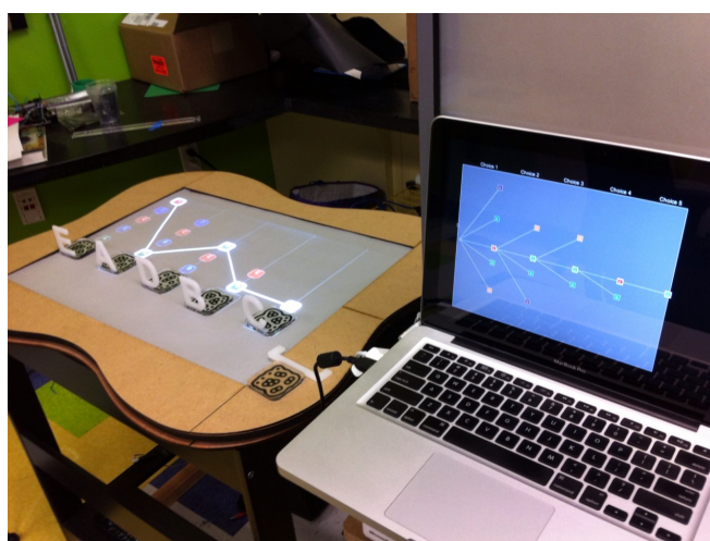
Figure 2.25: Combinatorix: tokens control a tabletop display (left) and a probability tree (right screen).
