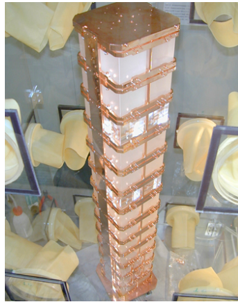
Figure 1.19 – The CUORE-0 tower with 52 \text{TeO}_2 crystals.
