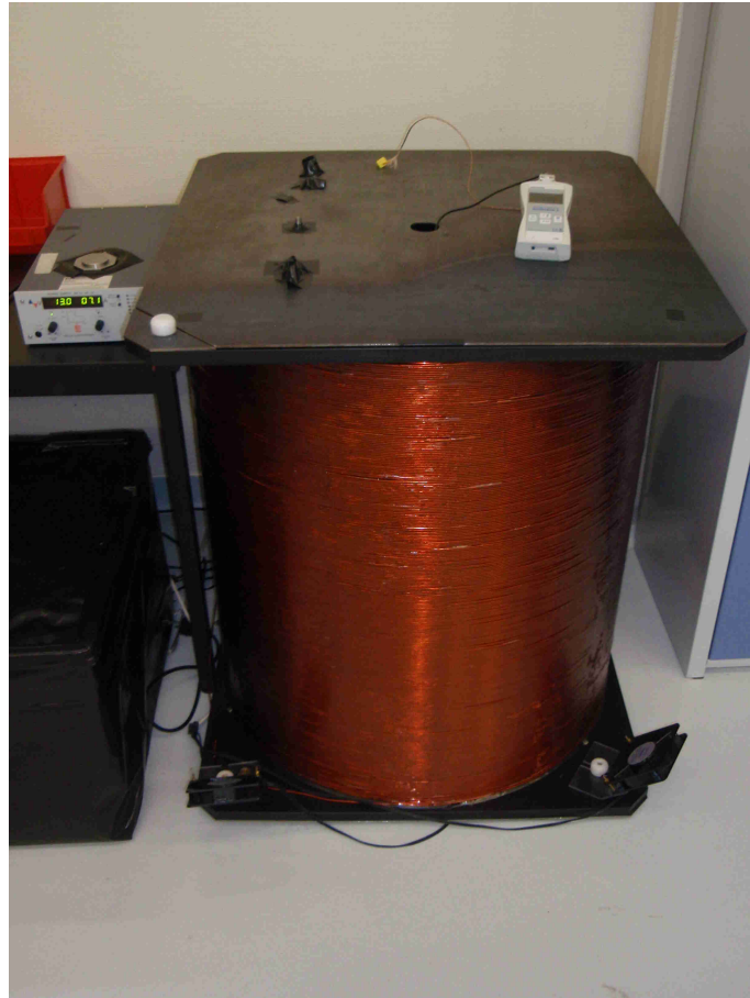
Figure 4.8 – The magnetic coil built in LAL to test the magnetic shieldings properties.
