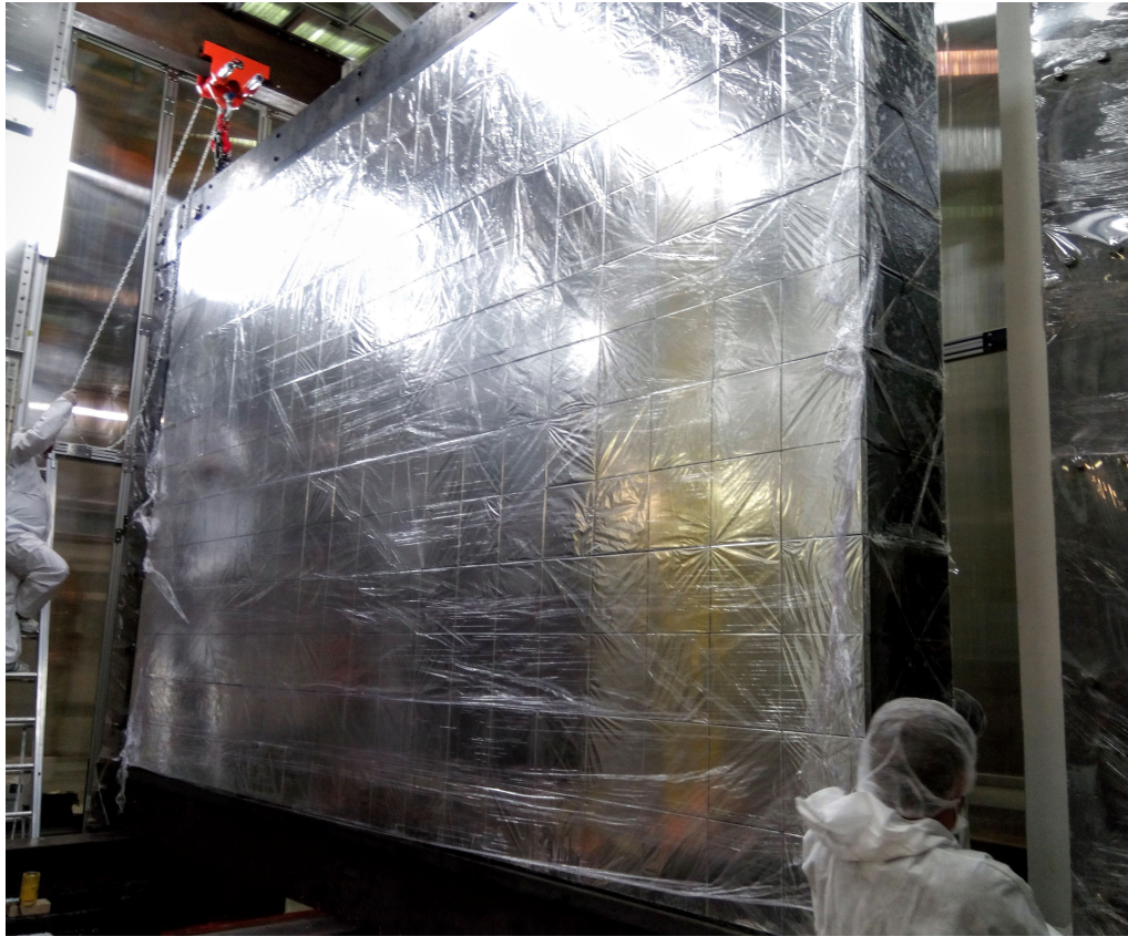
Figure 2.8 – One of the two calorimeter main walls assembled in LSM.
