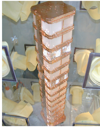
Figure 1.19 – The CUORE-0 tower with 52 \text{TeO}_2 crystals.
