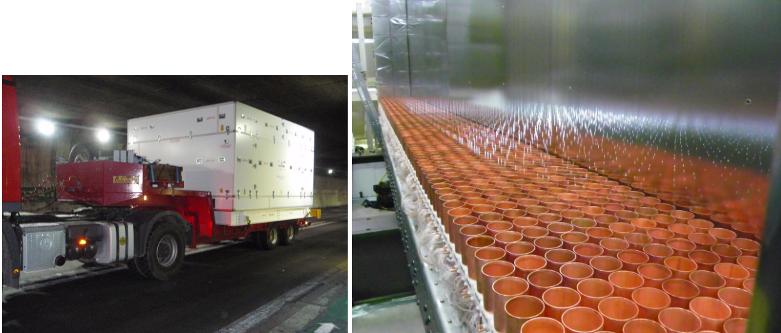
Figure 2.15 – (left) Delivery of a tracker C-section to LSM in its special transport box. (right) A full tracker module assembled in LSM. The nine layers of wires and the cathode rings are visible.
