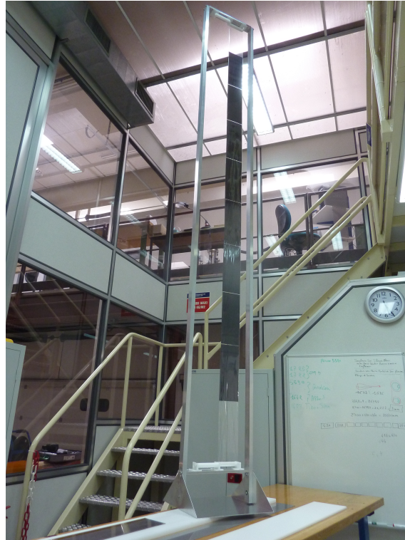
Figure 2.17 – A source strip made up of several selenium pads.
