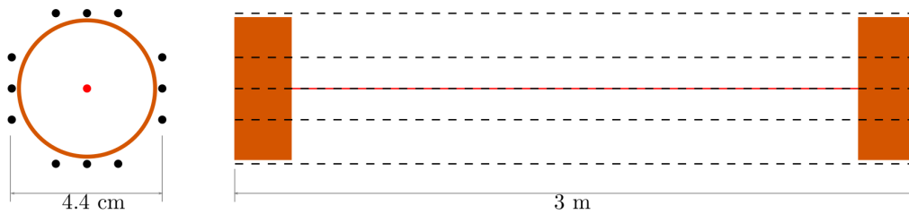
Figure 2.12 – Sketch of a SuperNEMO Geiger cell. ( left ) Transverse view: the anode wire is drawn in the center and the 12 field shaping wires are all around. ( right ) Side view: the anode is drawn in red in the center, the field wires are the dashed lines and the copper rings appear in red on both ends of the cell [56].
