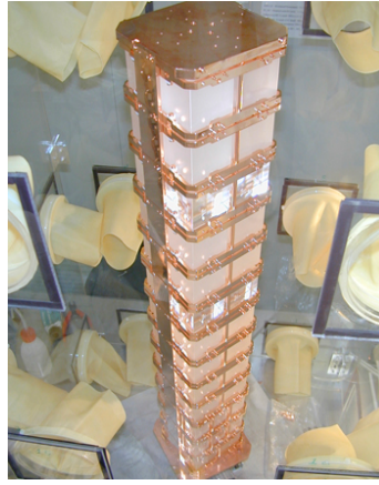
Figure 1.19 – The CUORE-0 tower with 52 \text{TeO}_2 crystals.
