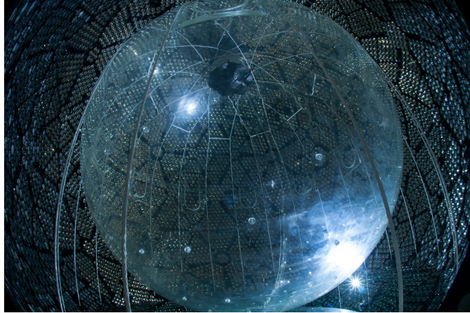
Figure 1.25 – Photo of the SNO+ detector. The acrylic vessel can be seen in the center with the PMTs all around [51].
