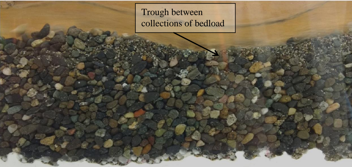
Figure 5.7 Image from the SLR camera of a trough forming during the SFU nat Experiment S.17 ( D_f=0.6 mm, fine feed/total feed = 42 %). Flow from left to right.
