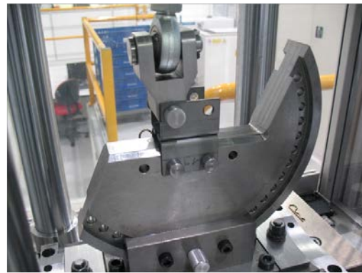
(b) Zoom on peeling load at an angle of 0^\circ/0^\circ .
