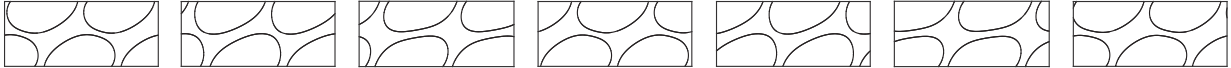
FIGURE 3. Temporal evolution of the bubble configuration for Ca = 0.1 , Bi = 0.1 and Pe = 1 (case B in table 1). Lines corresponds to the liquid-gas interface, i.e. \phi = 0 . The first snapshot corresponds to \tilde{t} = 1.82 and the time interval between two successive snapshots is \Delta\tilde{t} = 0.19 .
