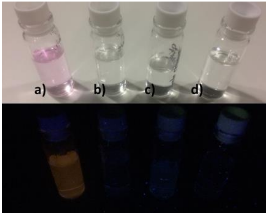
Fig. 3.21 Pictures of the solutions under ambient light and UV. a) initial dye solution ( 5 \cdot 10^{-7} M); b) dye solution filtered by cross-linked functionalized silica gel 60; c) dye solution filtered by cross-linked functionalized SBA-15; d) water without dye.
