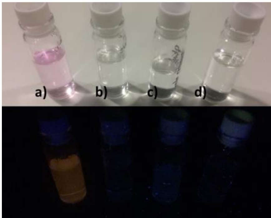
Fig. 3.21 Pictures of the solutions under ambient light and UV. a) initial dye solution ( 5 \times 10^{-7} M); b) dye solution filtered by cross-linked functionalized silica gel 60; c) dye solution filtered by cross-linked functionalized SBA-15; d) water without dye.
