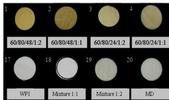
Figure 8: Colour development in samples treated under different experimental conditions. WPI means whey protein isolate and MD means maltodextrin. Numbers correspond to the reaction conditions: temperature ( ^\circ\text{C} )/ relative humidity (%)/ time (h)/ and molar ratio, respectively (Martinez-Alvarenga et al. 2014)
