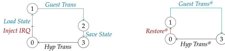
FIGURE 5.2: Correspondence between Transitions of the Concrete Level (left) and the Abstract Level (right)
