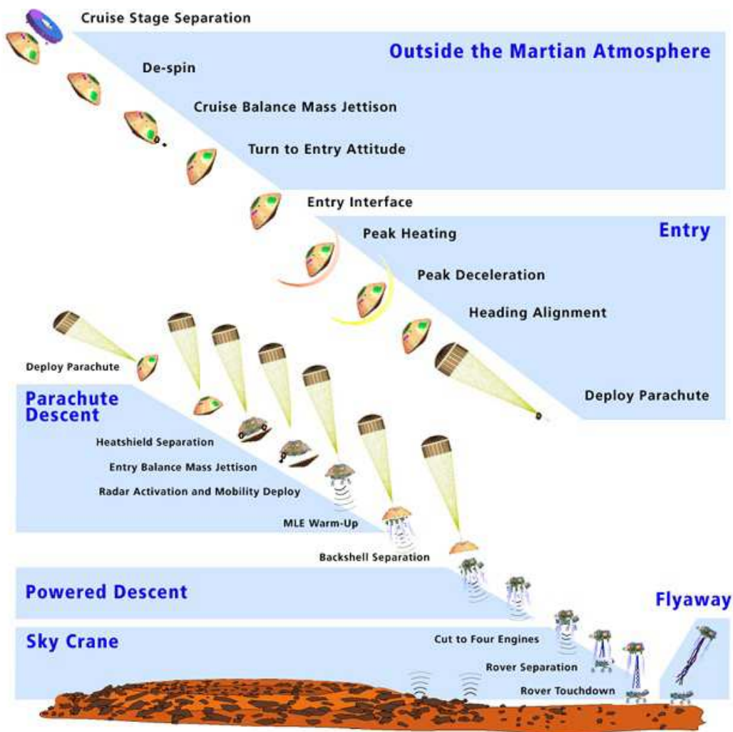
Figure 1.1.: Entry, Descent, and Landing sequence for the Mars Science Laboratory (source: NASA/JPL).
