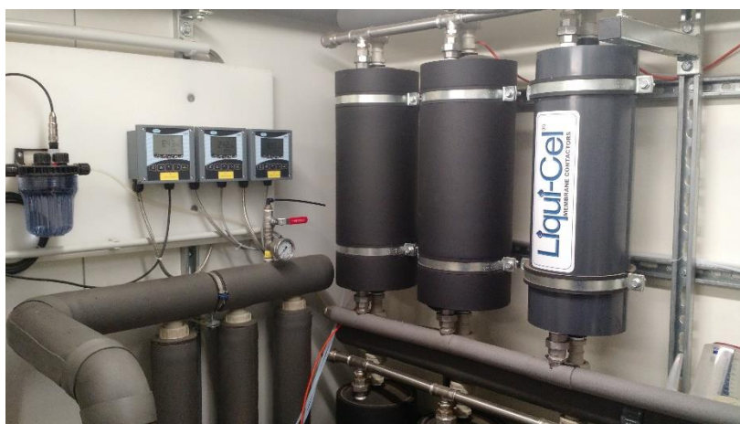
Figure 1.19 – Small scale biogas upgrading unit using hollow fiber membrane contactors Plant capacity: 6 \text{ Nm}_{\text{CH}_4}^3 \cdot \text{h}^{-1} - Germany
