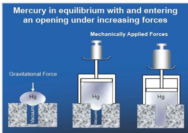
Figure 2.1– Mercury intrusion porosimetry principle (source: Micromeritics)
