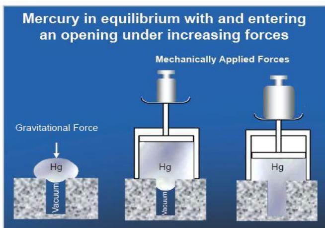
Figure 2.1– Mercury intrusion porosimetry principle
